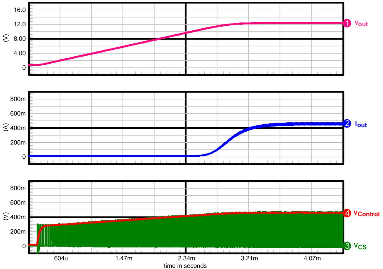
Figure 4. Startup Simulation showing the Natural Soft-start
