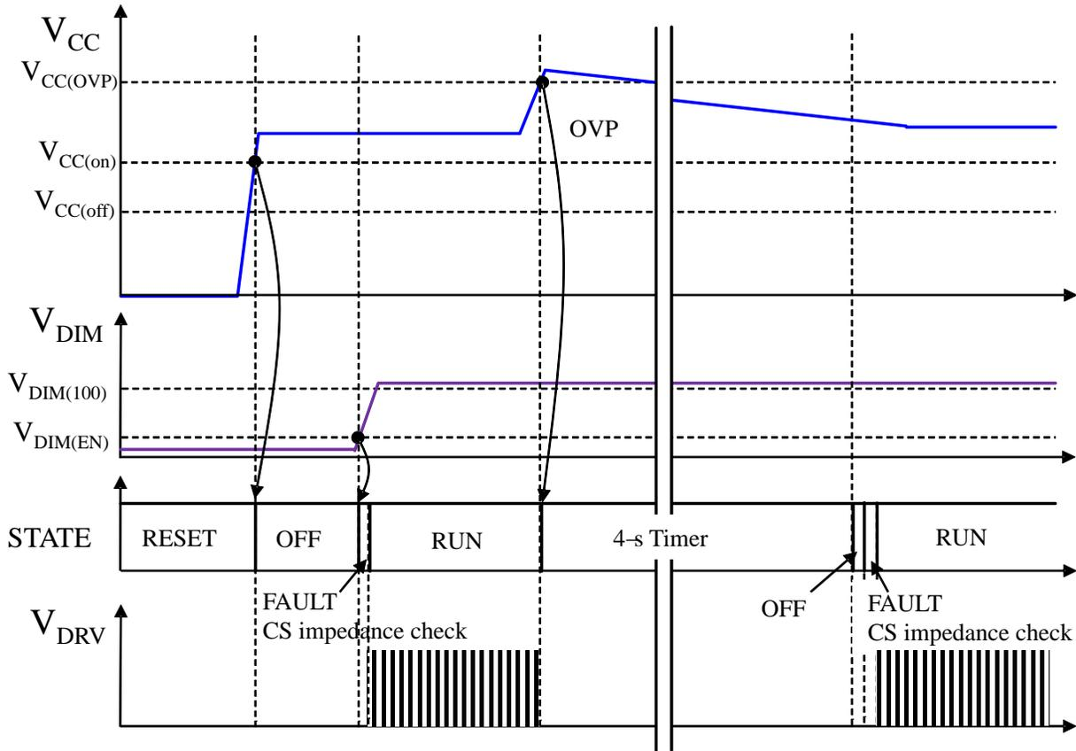
Figure 9. V<sub>CC</sub> Over Voltage Protection Chronograms
