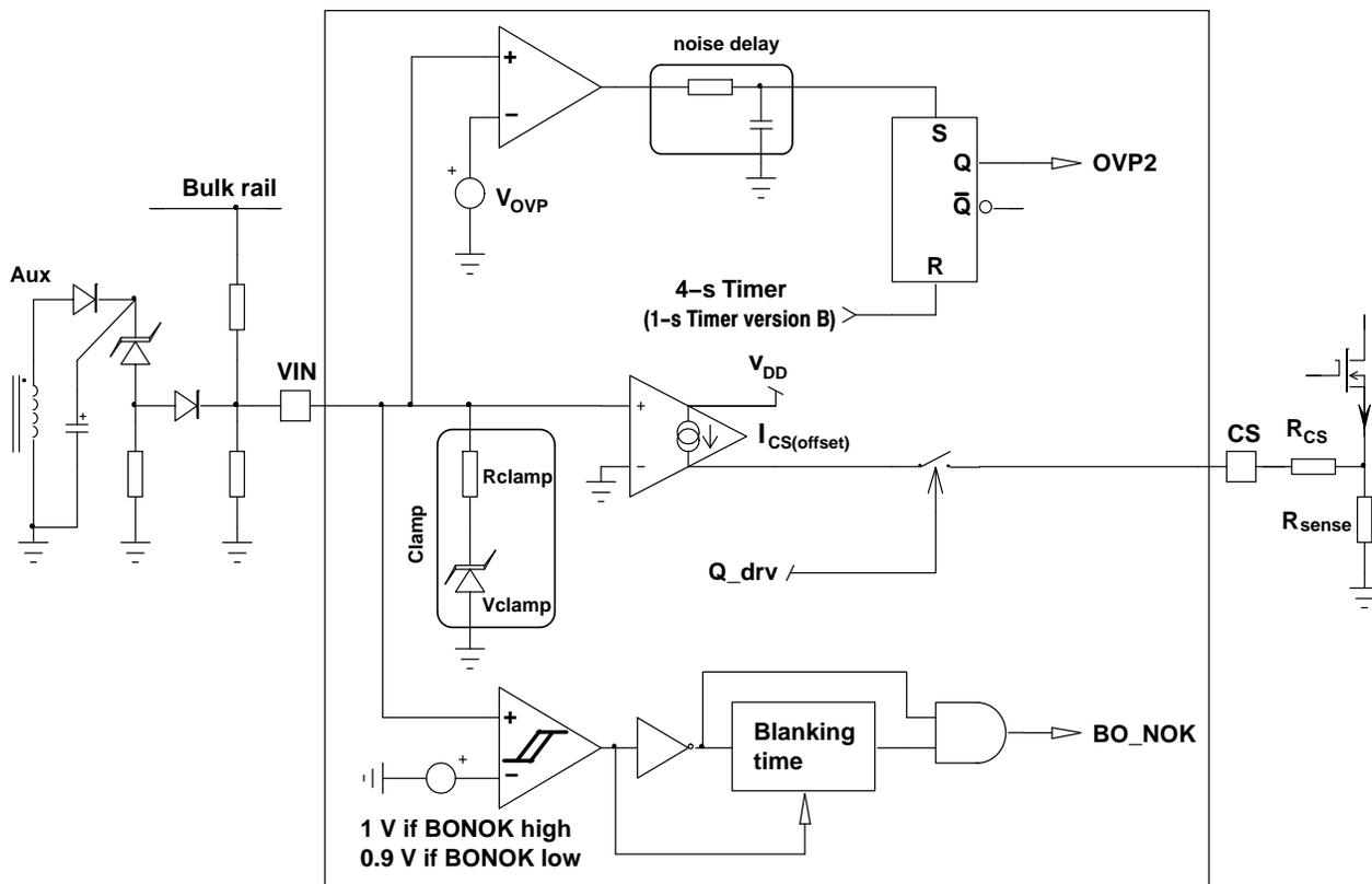
Figure 12. Line Feed-Forward, Adjustable OVP and Brown-out Schematic
