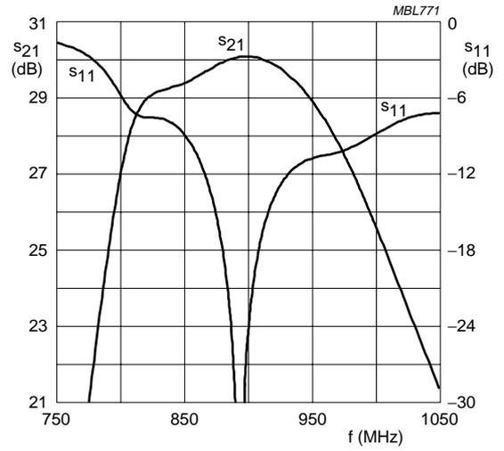
Fig.11 s-parameters as a function of frequency.
