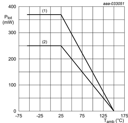
(1) FR4 PCB, single-sided, 35 μm copper, tin-plated, mounting pad for collector 1 cm<sup>2</sup>
