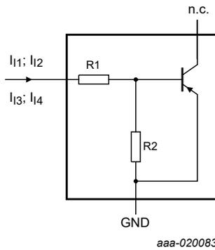
Fig. 10. Resistor test circuit
