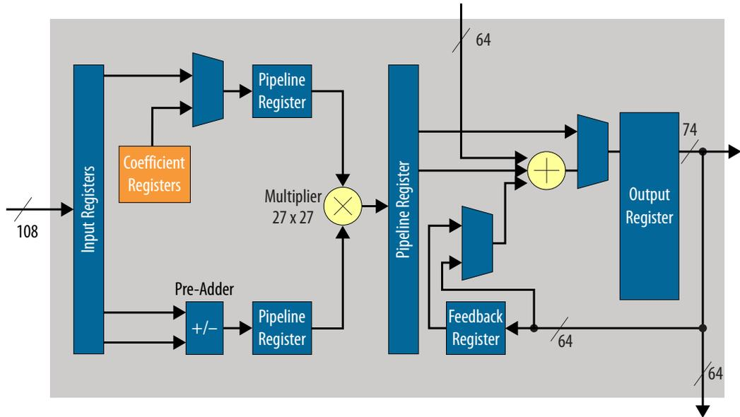
**Figure 14. DSP Block: Single Precision Floating Point Mode**
