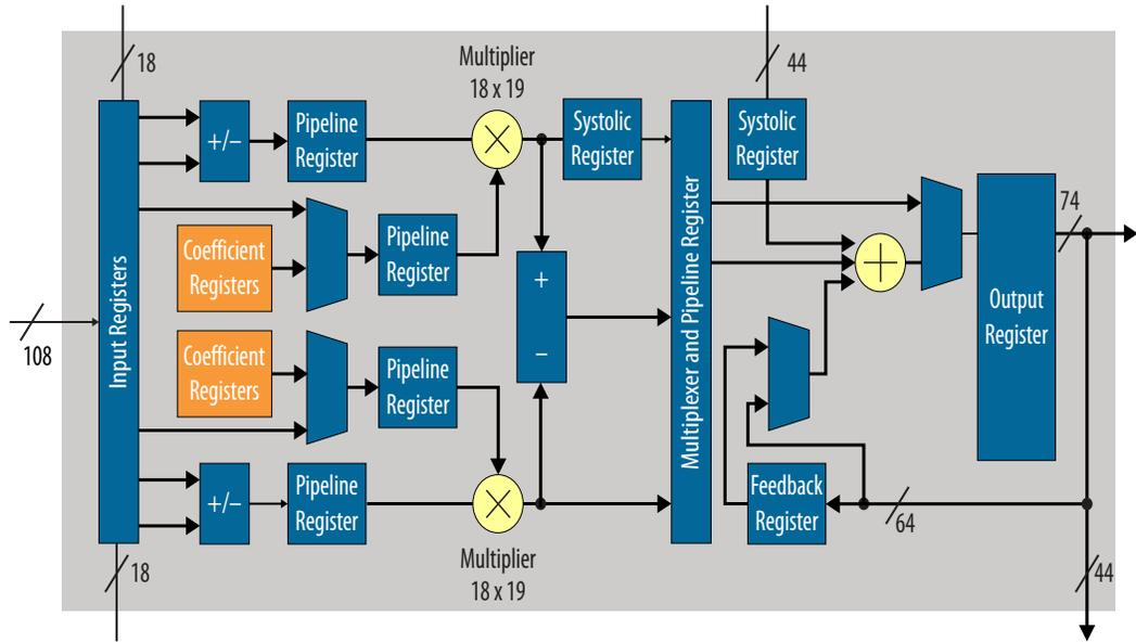
**Figure 13. DSP Block: High Precision Fixed Point Mode**
