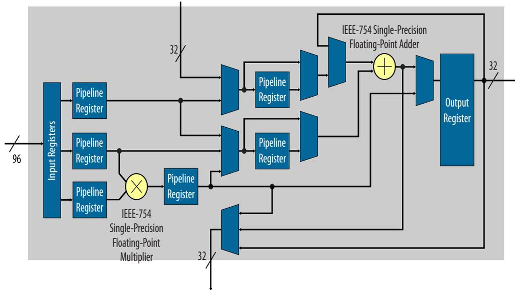
Each DSP block can be independently configured at compile time as either dual 18x19 or a single 27x27 multiply accumulate. With a dedicated 64 bit cascade bus, multiple variable precision DSP blocks can be cascaded to implement even higher precision DSP functions efficiently.
