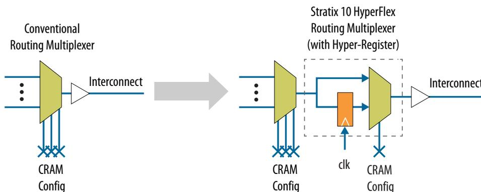
The Hyper-Registers enable the following key design techniques to achieve the 2X core performance increases:
