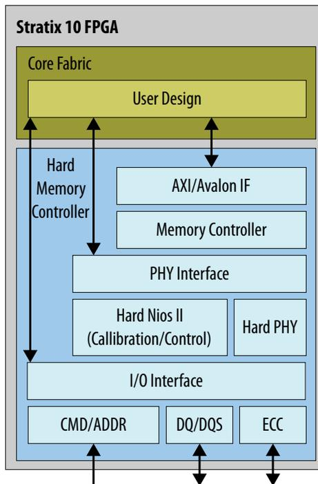
Each I/O bank contains 48 general purpose I/Os and a high-efficiency hard memory controller capable of supporting many different memory types, each with different performance capabilities. The hard memory controller is also capable of being bypassed and replaced by a soft controller implemented in user logic. The I/Os each have a hardened double data rate (DDR) read/write path (PHY) capable of performing key memory interface functionality such as:
