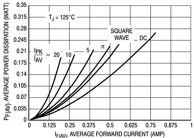
**Figure 6. Power Dissipation**
