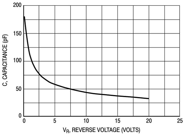
**Figure 3. Typical Capacitance**
