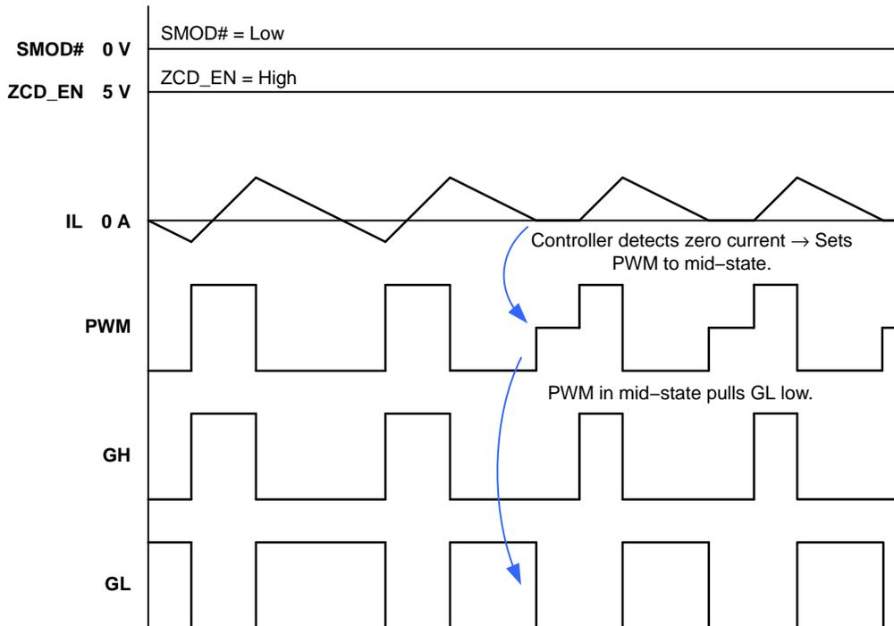
**Figure 10. Timing Diagram – 3-state PWM Controller, with ZCD**
