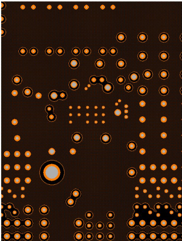
Figure 14. Layer 2 Copper Layer (Ground Plane)
