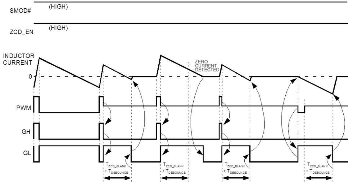
**Figure 9. Timing Diagram – 3-state PWM Controller, No ZCD**
