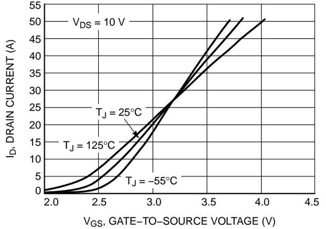
Figure 2. Transfer Characteristics
