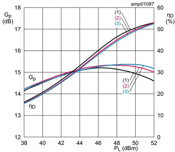
$V_{DS} = 30\text{ V}; I_{Dq} = 370\text{ mA}; V_{GS(amp)peak} = 0.85\text{ V}.$
