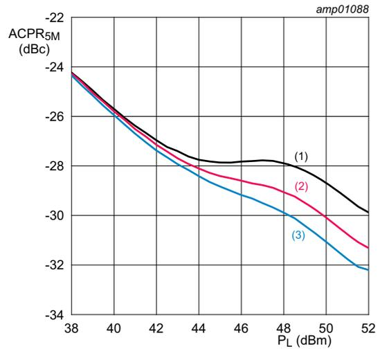
$V_{DS} = 30\text{ V}; I_{Dq} = 370\text{ mA}; V_{GS(amp)peak} = 0.85\text{ V}.$
