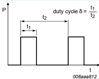
Fig. 17. Duty cycle definition
