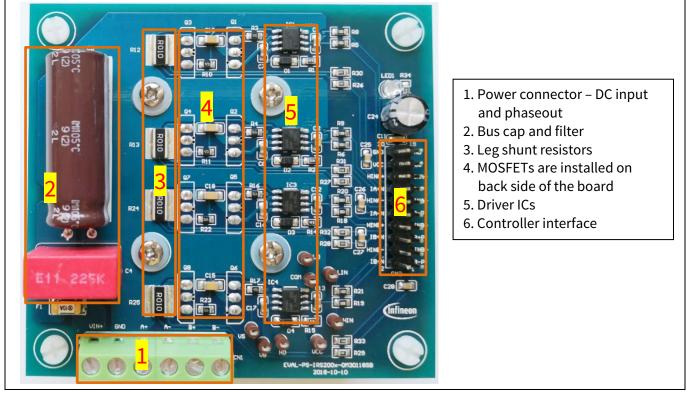
Figure 2 Top view of the EVAL-PS-IRS200x-OM30118SB
