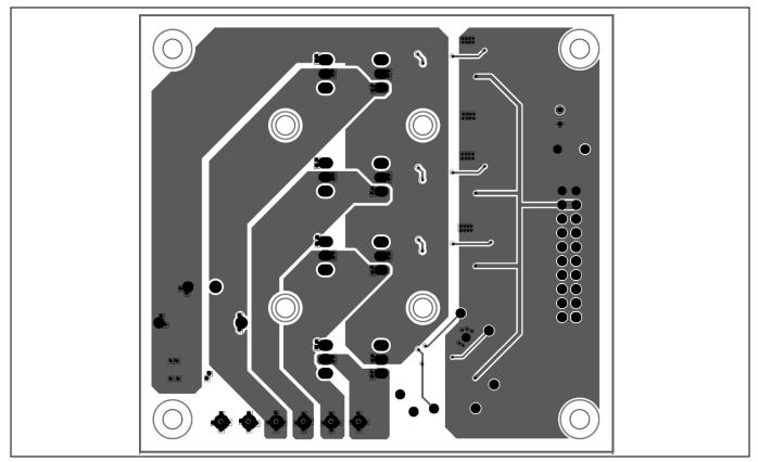
Figure 15 Bottom layer routing of the EVAL-PS-IRS200x-OM30118SB
