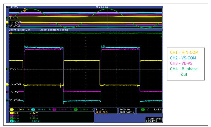
Figure 8 The Vs signal probed at 7 A<sub>RMS</sub> phase-out current
