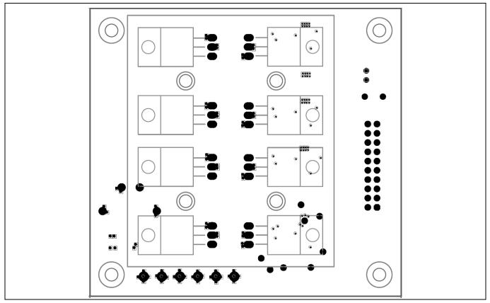
Figure 14 Bottom assembly drawing of the EVAL-PS-IRS200x-OM30118SB
