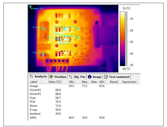
Figure 9 Thermal breakdown at 72 V<sub>DC</sub> input and 7 A<sub>RMS</sub> phase current
