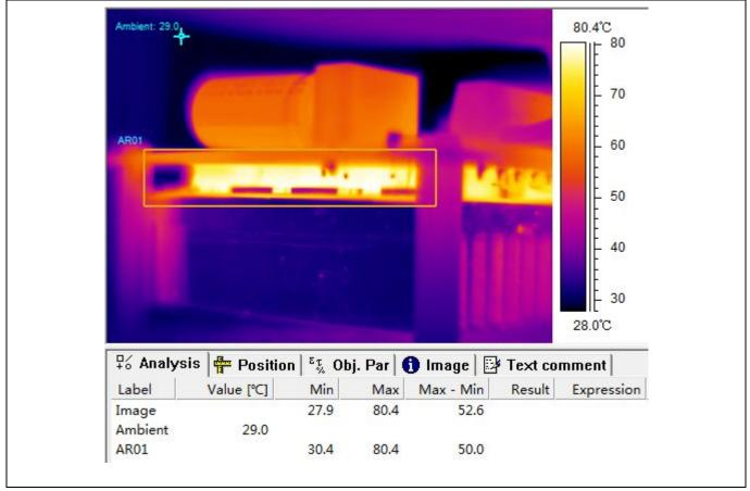
Figure 10 MOSFET temperature rise at 72  $V_{\text{DC}}$  input and 7  $A_{\text{RMS}}$  phase current
