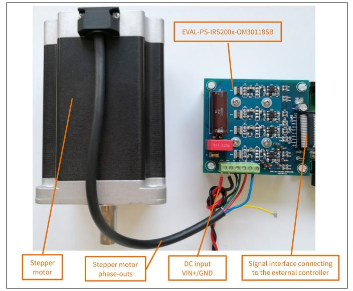
Figure 6 System configuration for running a stepper motor
