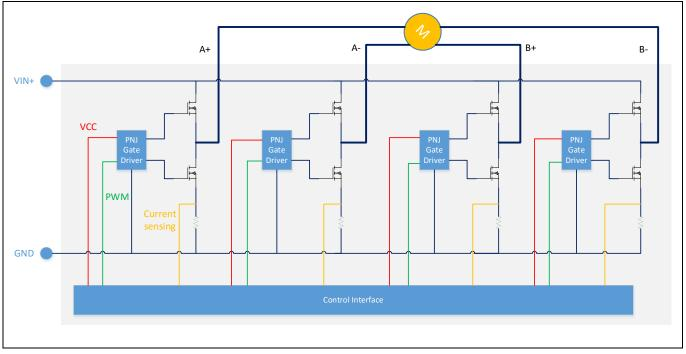
Figure 1 Block diagram of the EVAL-PS-IRS200x-OM30118SB
