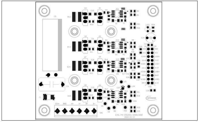
Figure 12 Top assembly drawing of the EVAL-PS-IRS200x-OM30118SB
