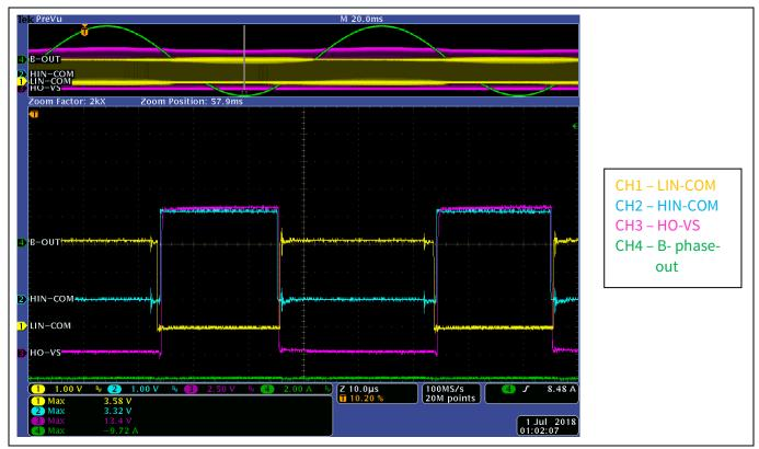
Figure 7 The input signals probed at 7 ARMS phase-out current
