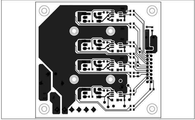
Figure 13 Top layer routing of the EVAL-PS-IRS200x-OM30118SB
