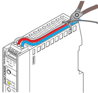
Figure 11 Shorten protruding ends of the cable binder
