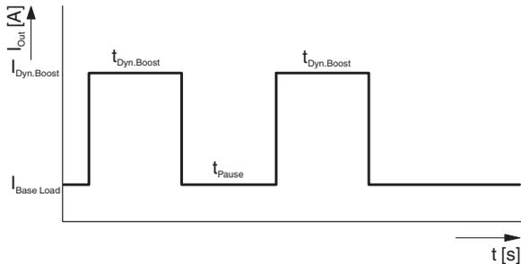
Figure 17 Basic curve of the dynamic boost process
