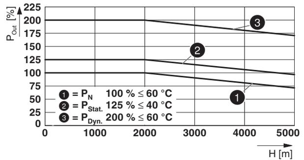
Figure 30 Output power depending on the installation height
