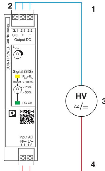
Figure 1 Potential-related wiring for the high-voltage test
