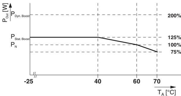
Figure 29 Output power depending on the ambient temperature
