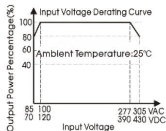
1. With an AC input between 85 -100VAC/277- 305VAC and a DC input between 70 - 120VDC/390 - 430VDC, the output power must be derated as per temperature derating curves;
