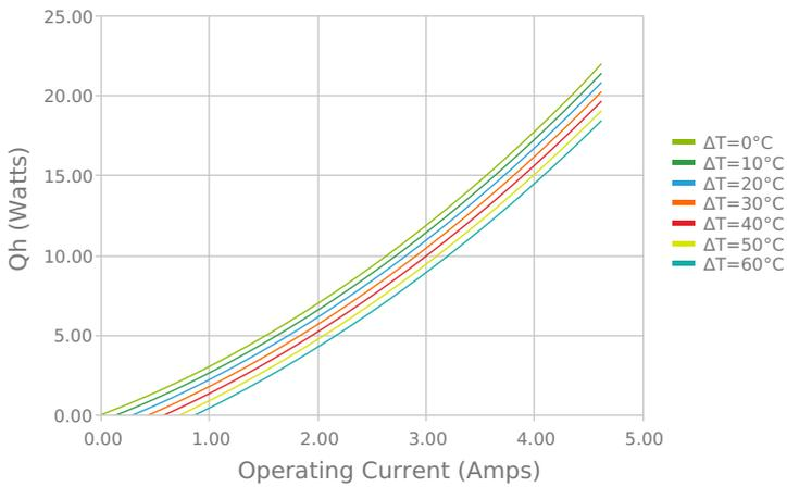
Total Heat Dissipated at Hot Side (Qh=Qc+Pin)
