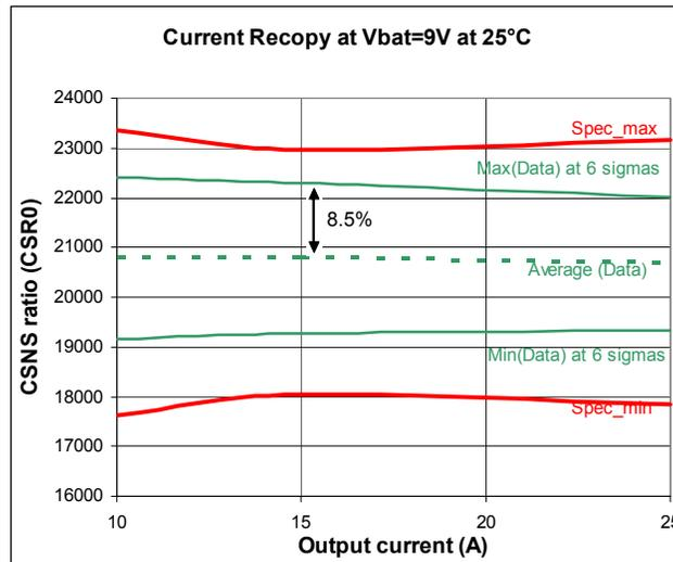
Figure 14. CSR0 Ratio Deviation in Function Manufacturing
