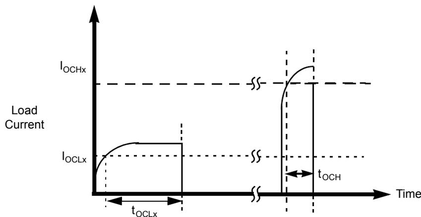
**Figure 5. Overcurrent Shutdown**
