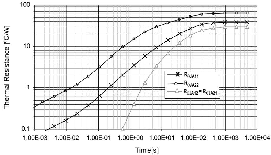
**Figure 18. Transient Thermal Resistance  $R_{\theta JA}$  (1.0 W Step Response)
