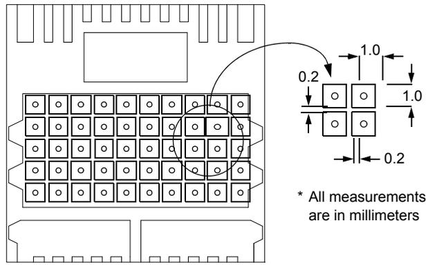
Note: Recommended via diameter is 0.5 mm. PTH (plated through hole) via must be plugged / filled with epoxy or solder mask in order to minimize void formation and to avoid any solder wicking into the via.
