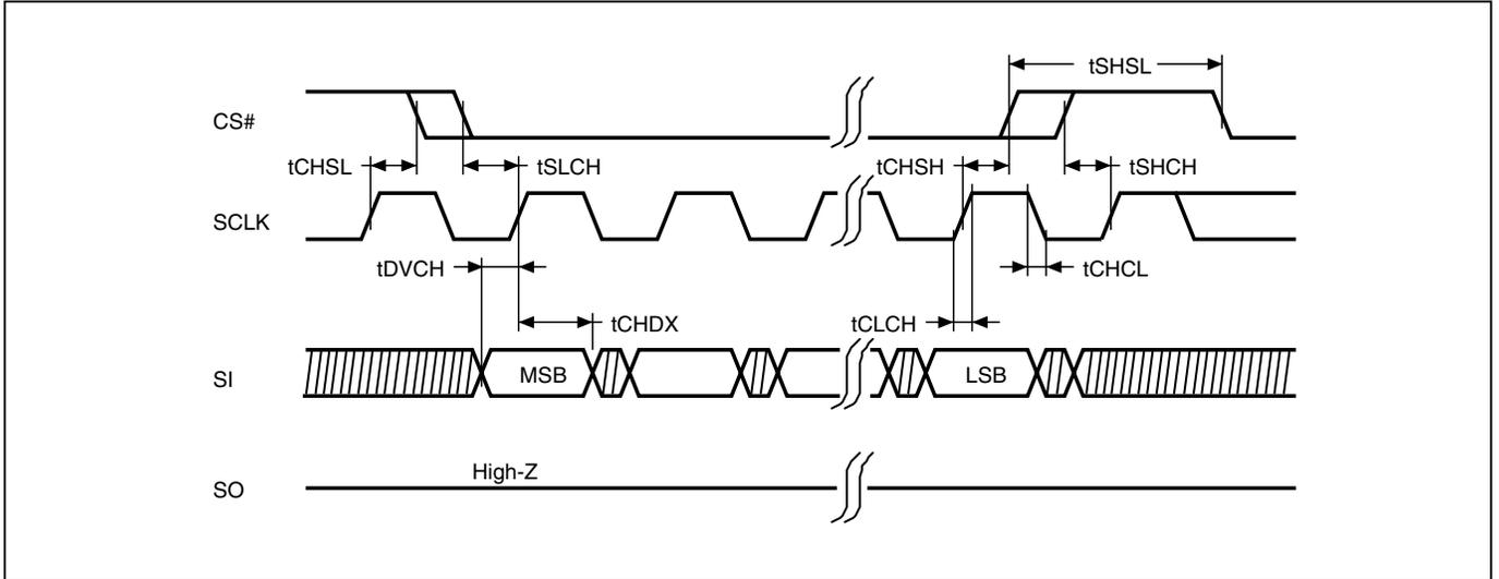
**Figure 6. Output Timing**
