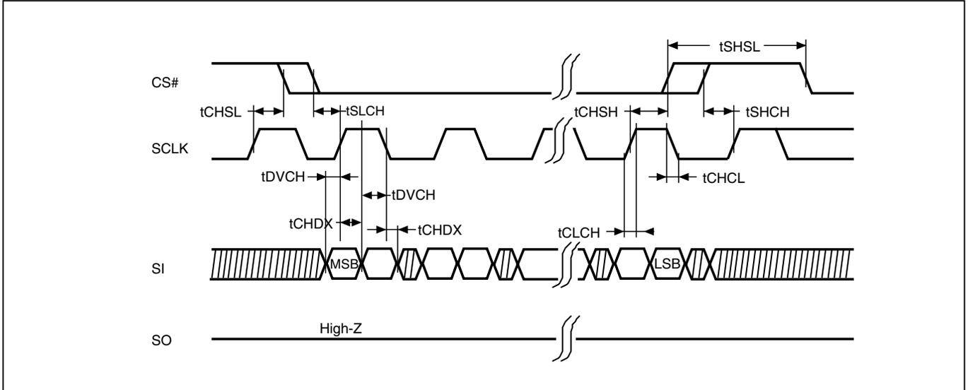
**Figure 8. Serial Output Timing for Double Transfer Rate Mode**
