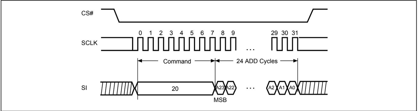
**Figure 27. Block Erase (BE/EB32K) Sequence (Command D8/52)**
