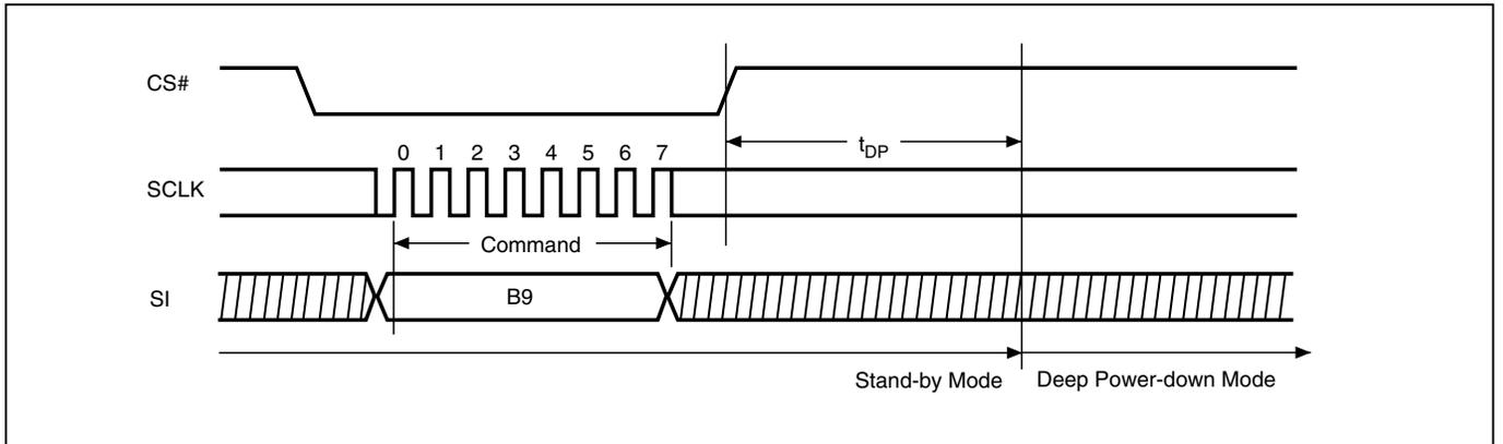
**Figure 33. Release from Deep Power-down and Read Electronic Signature (RES) Sequence (Command AB)**
