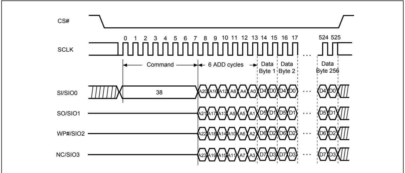
**Figure 31. Continuously Program (CP) Mode Sequence with Hardware Detection (Command AD)**
