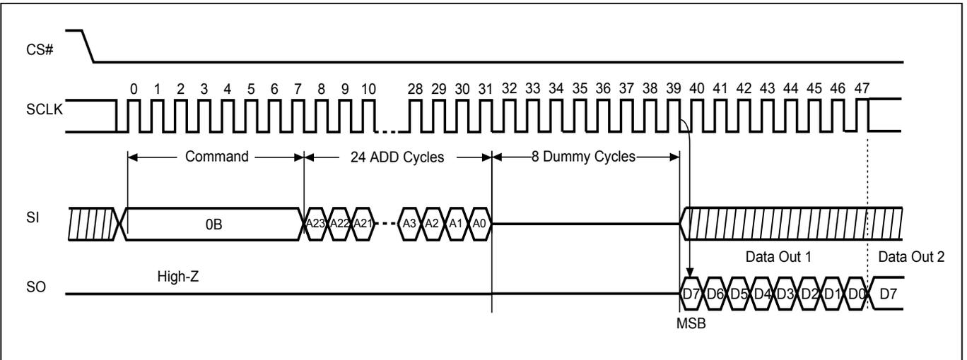
**Figure 17. Fast DT Read (FASTDTRD) Sequence (Command 0D)**
