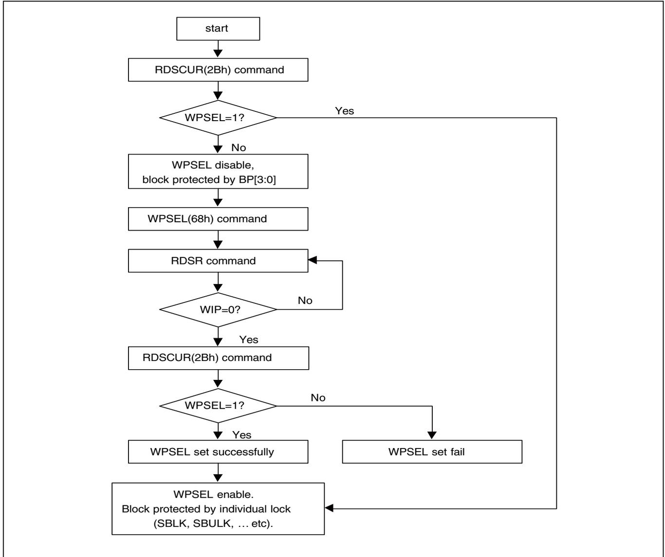
**(30) Single Block Lock/Unlock Protection (SBLK/SBULK)**
