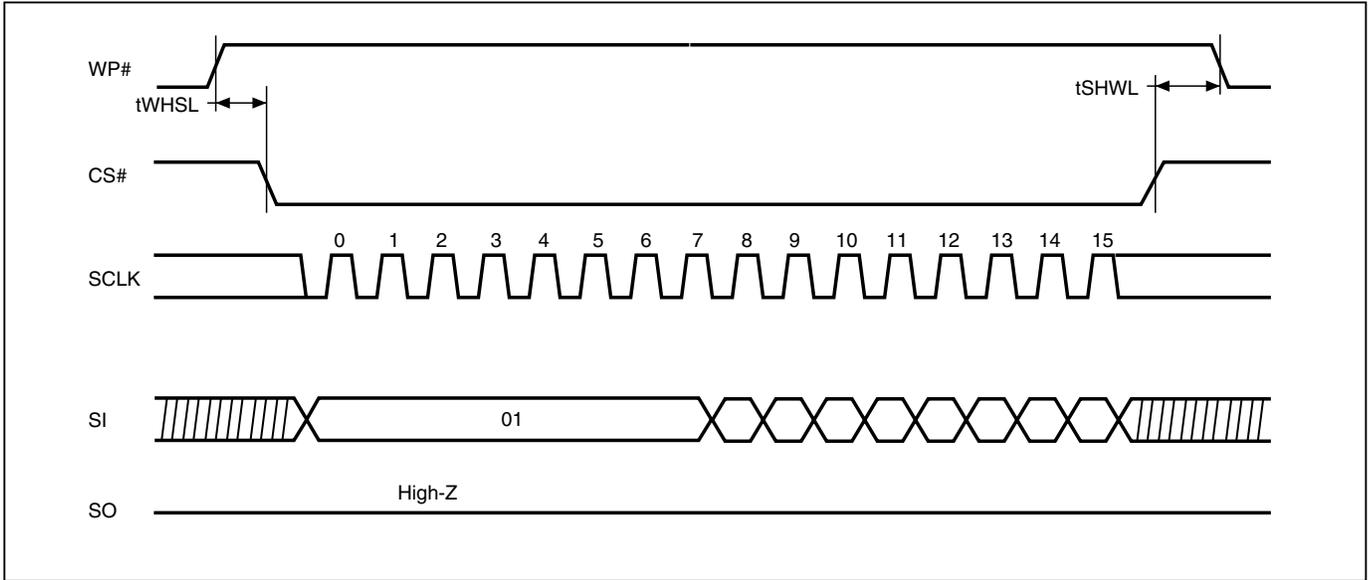
**Figure 10. Write Enable (WREN) Sequence (Command 06)**
