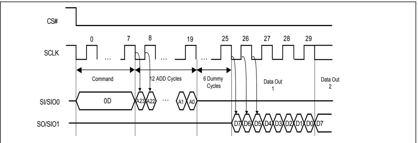
**Figure 18. 2 x I/O Read Mode Sequence (Command BB)**
