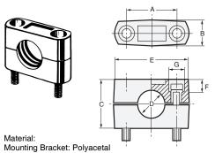
Hexagonal bolt and spring washer: Nickel-plated iron
