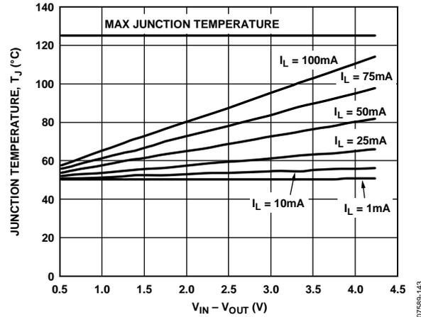
Figure 43. WLCSP, 500 mm<sup>2</sup> of PCB Copper,  $T_A = 50^\circ\text{C}$
