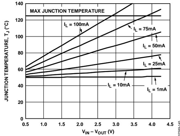
Figure 45. WLCSP, 0 mm<sup>2</sup> of PCB Copper,  $T_A = 50^\circ\text{C}$
