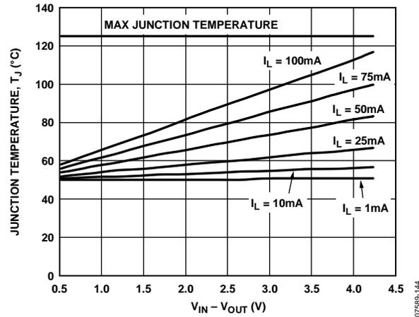
Figure 44. WLCSP, 100 mm<sup>2</sup> of PCB Copper,  $T_A = 50^\circ\text{C}$
