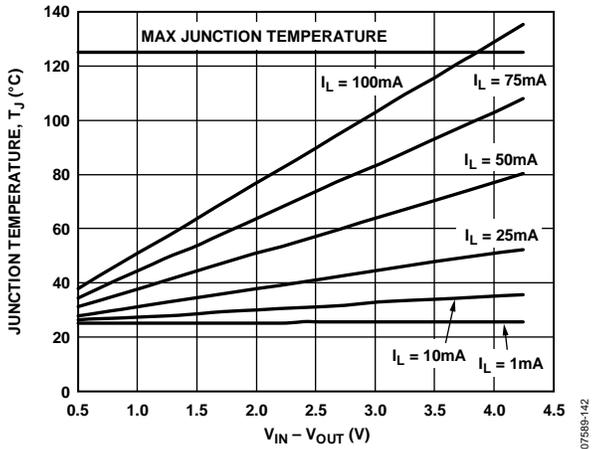
Figure 42. WLCSP, 0 mm<sup>2</sup> of PCB Copper,  $T_A = 25^\circ\text{C}$
