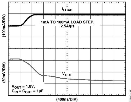
Figure 28. Output Transient Response,  $C_{OUT} = 1 \mu\text{F}$
