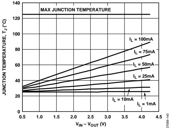
Figure 40. WLCSP, 500 mm<sup>2</sup> of PCB Copper,  $T_A = 25^\circ\text{C}$
