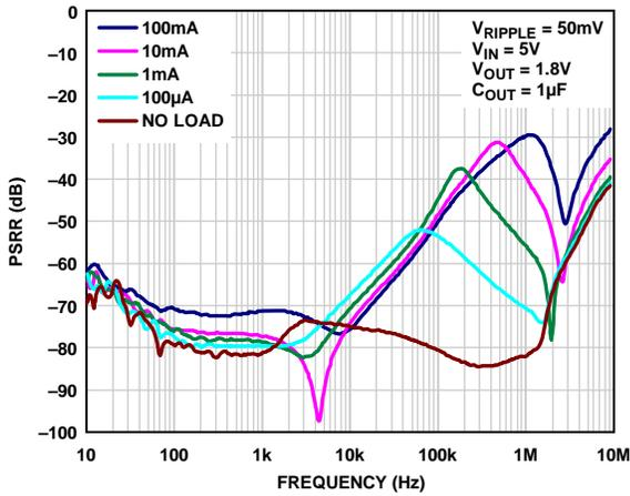
Figure 18. Power Supply Rejection Ratio vs. Frequency
