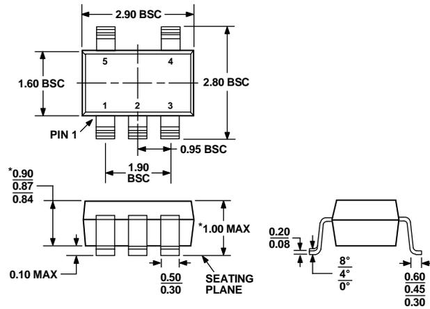
\*COMPLIANT TO JEDEC STANDARDS MO-193-AB WITH THE EXCEPTION OF PACKAGE HEIGHT AND THICKNESS.
