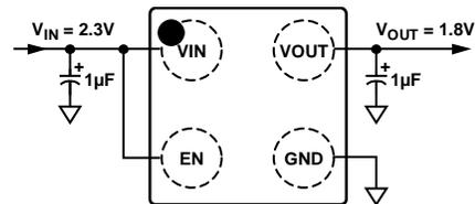
Figure 2. ADP120 WLCSP with Fixed Output Voltage, 1.8 V
