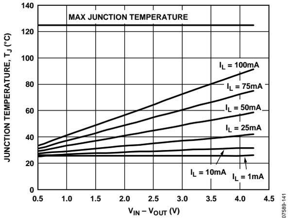
Figure 41. WLCSP, 100 mm<sup>2</sup> of PCB Copper,  $T_A = 25^\circ\text{C}$
