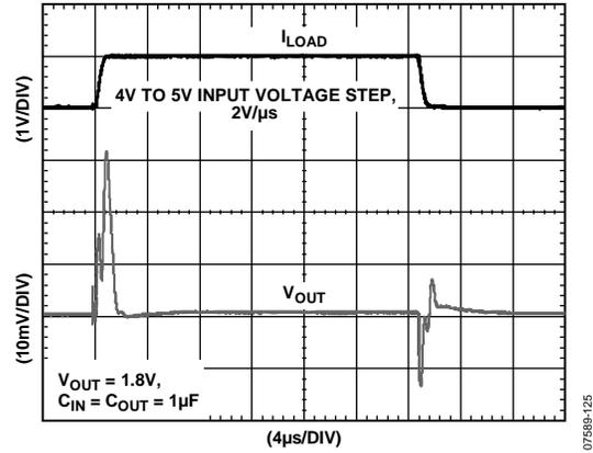
Figure 25. Line Transient Response, Load Current = 100 mA
