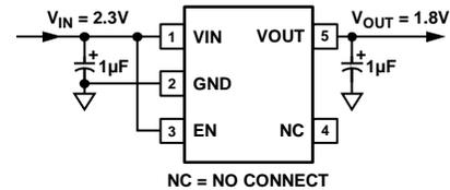
Figure 1. ADP120 TSOT with Fixed Output Voltage, 1.8 V
