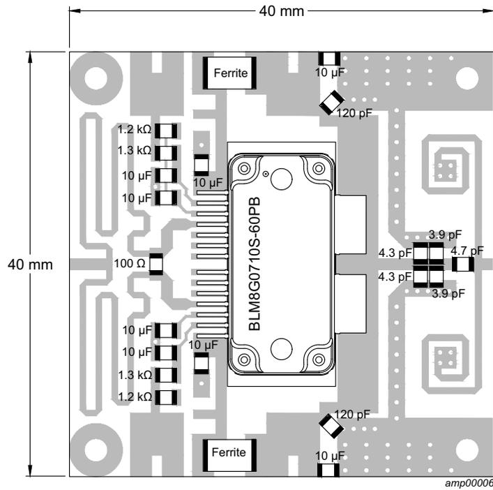
Printed-Circuit Board (PCB): Rogers 4350; thickness = 0.508 mm.
