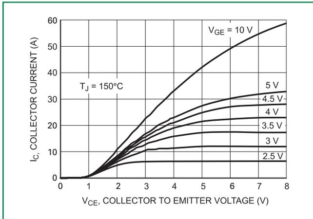
**Figure 4. Transfer Characteristics**
