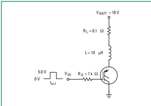
**Figure 18. Circuit Configuration for Short Circuit Test #2**
