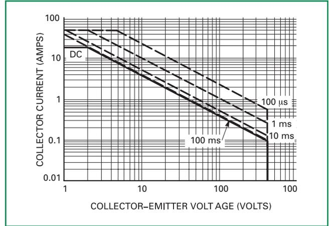
**Figure 15. Pulse Train Safe Operating Area**
