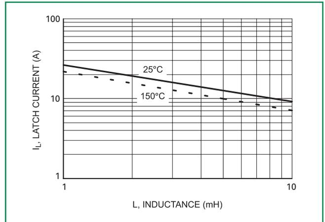
Figure 11. Typical Open Secondary Latch Current vs. Inductance
