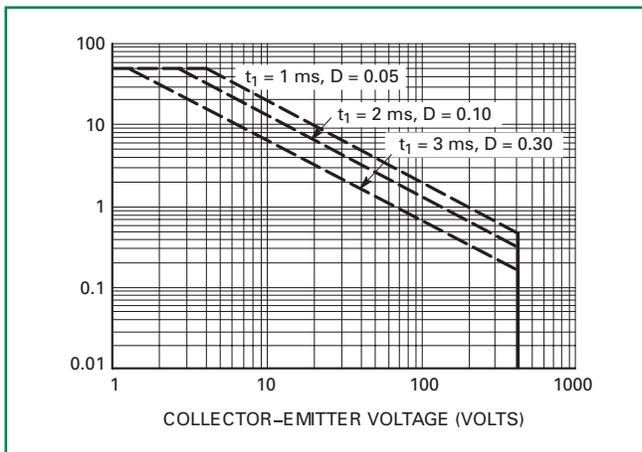
**Figure 16. Pulse Train Safe Operating Area**
