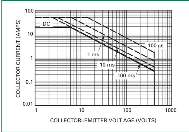
**Figure 14. Single Pulse Safe Operating Area**
