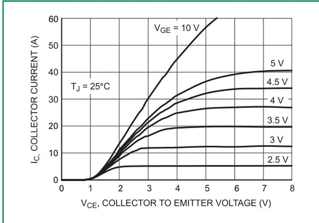
**Figure 2. Output Characteristics**
