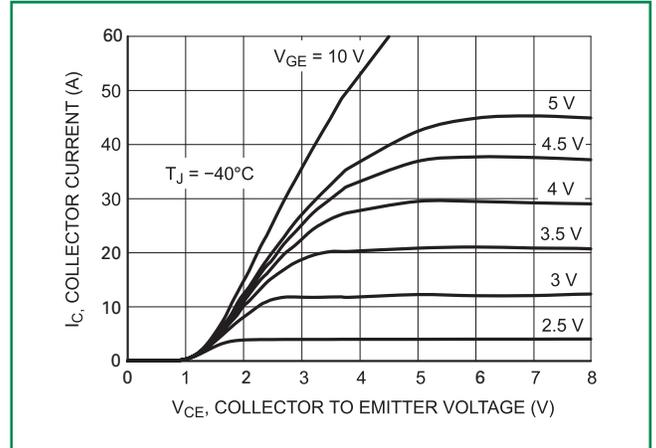
**Figure 3. Output Characteristics**
