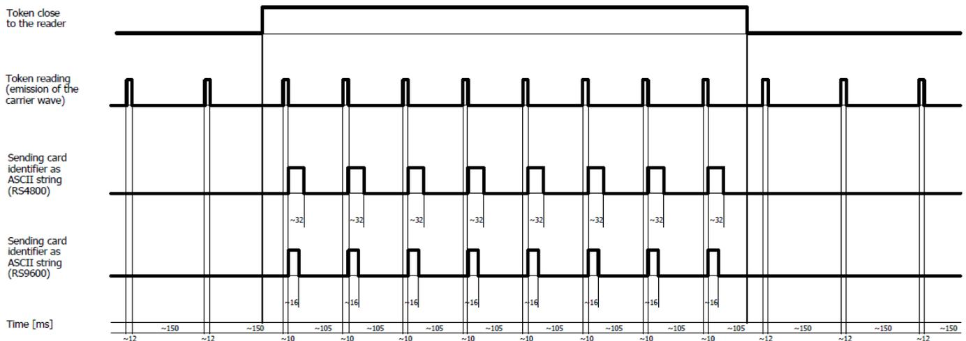
1. The reader is waiting for the proximity of the token (card) trying to read it at a frequency of about 6 times per second ( $\sim 12$  ms [checking the presence of the card] +  $\sim 150$  ms [gap between successive checks]).
