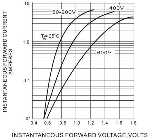
Fig. 1 FORWARD CHARACTERISTICS
