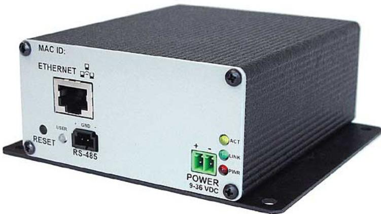
The EM1500 Serial-Ethernet Bridge is a device that converts multi-point serial communications to a TCP/IP network. The EM1500 connects to and network enables as many as 4 RS-232 serial devices simultaneously. In addition, the EM1500 provides an SPDT relay, 2 digital open collector outputs and 3 digital inputs suitable for interfacing to mechanical switches or logic level circuits.
