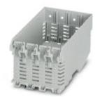
DIN rail housing, Lower housing part with metal foot catch, with vents, width: 75.9 mm, cross connection: DIN rail connector (optional), number of positions cross connector: 8, color: light gray (7035)
