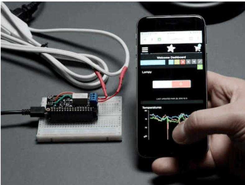
There are two 'flavors' of these FeatherWings, the first is the simple **Non-Latching** relay. This Wing has a single Set pin. Normally, the **COM** pin is connected mechanically to the **NC** pin and the **NO** pin is disconnected.
