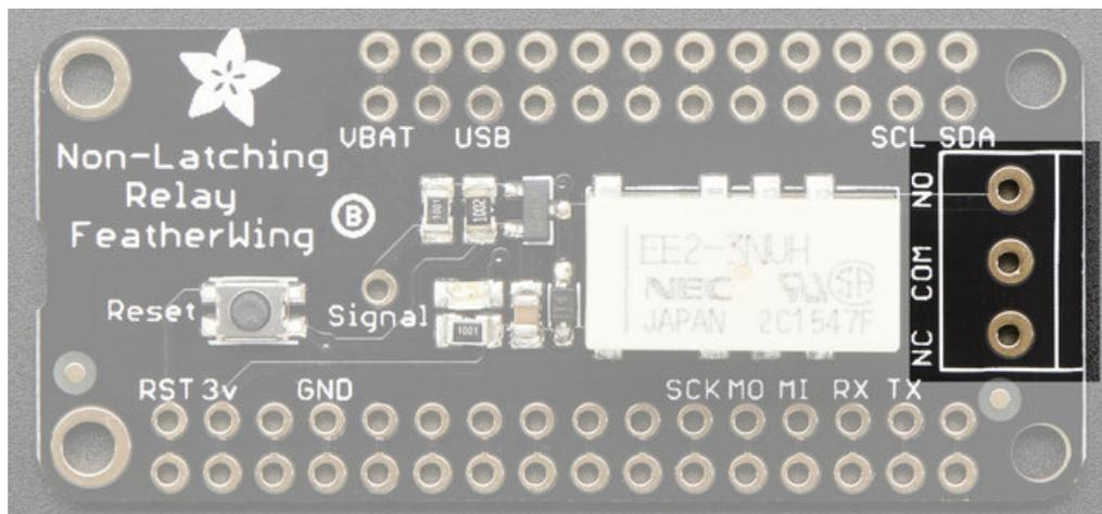
Both Wings have the same output, a 3-pin 3.5mm terminal block. The **COM** pin is what you should connect the signal you're planning to switch. If the relay is unset, the **NC** pin (Normally Connected) is mechanically connected to **COM**. **NO** (Normally Open) is mechanically disconnected.
