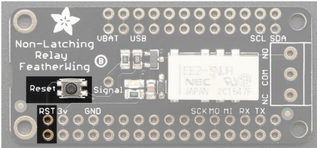
There is a Reset button on both Wings, this is connected to the **RST** pin and will short it to ground. It is not connected to the relay at all, its handy for restarting your Feather
