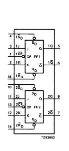
Fig.4 Functional diagram.
