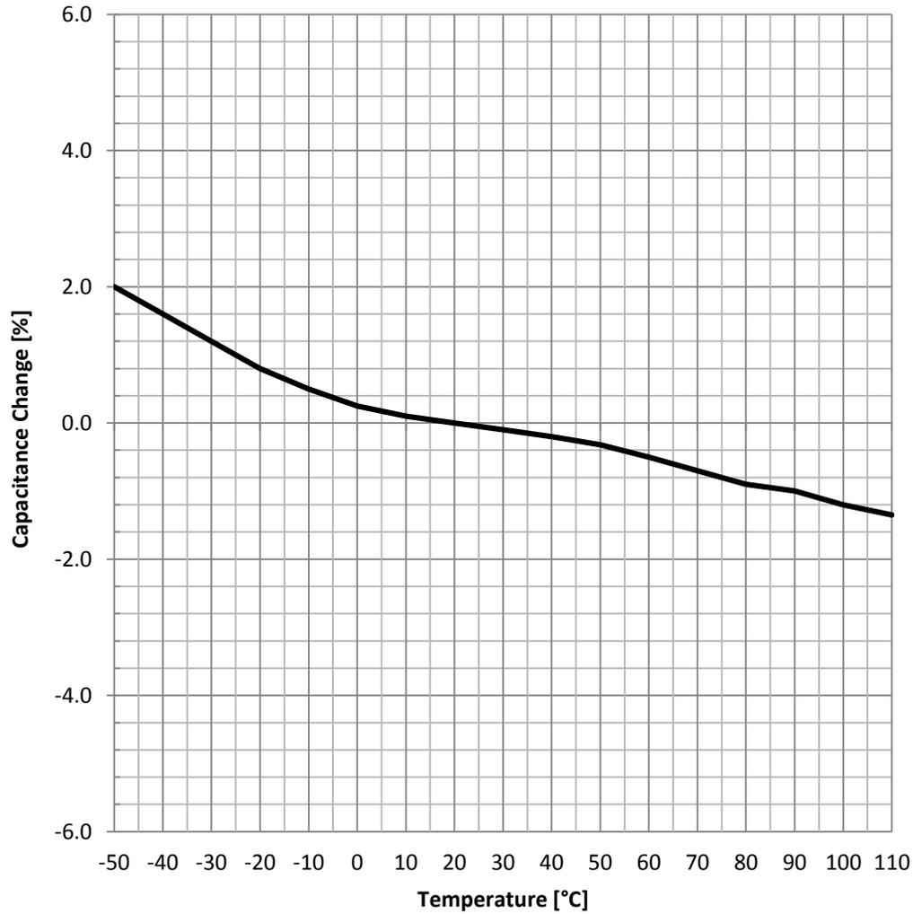
Test Equipment: E4991A or equivalent
