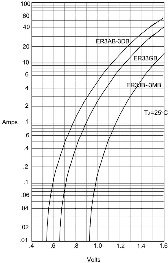
Instantaneous Forward Current - Amperes versus
