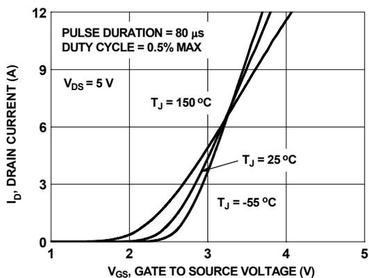
**Figure 5. Transfer Characteristics**
