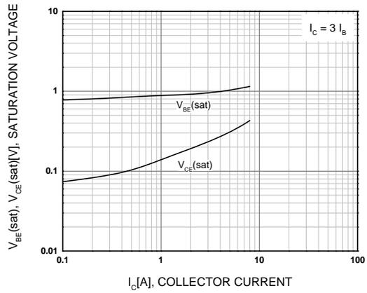
Figure 2. Saturation Voltage
