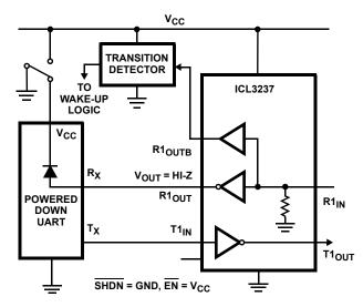
FIGURE 3. DISABLED RECEIVERS PREVENT POWER DRAIN
