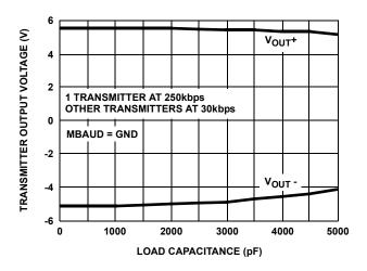
FIGURE 8. LOW SPEED TRANSMITTER OUTPUT VOLTAGE
