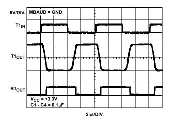
FIGURE 6. LOOPBACK TEST AT 250kbps (C<sub>L</sub> = 1000pF)
