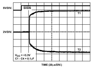
FIGURE 4. TRANSMITTER OUTPUTS WHEN EXITING POWERDOWN
