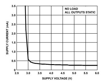
FIGURE 14. SUPPLY CURRENT vs SUPPLY VOLTAGE
