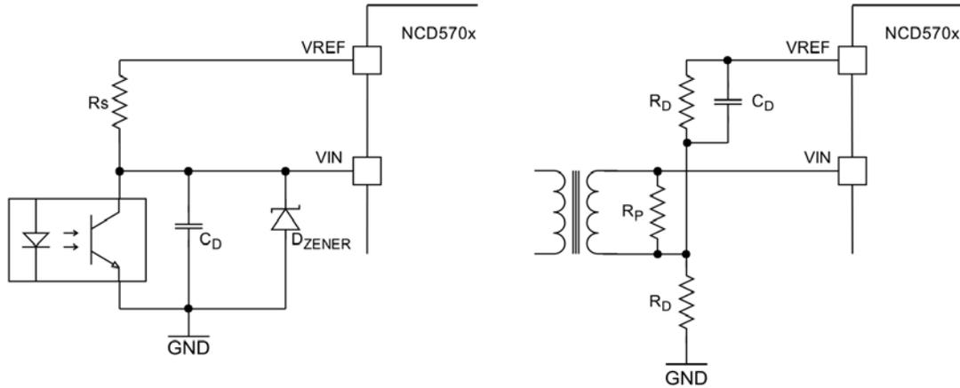
**Figure 28. Opto-coupler or Pulse Transformer At Input**
