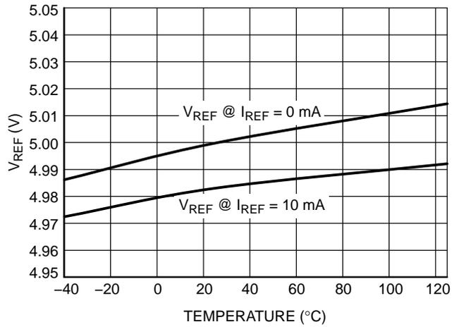
Figure 11. V<sub>REF</sub> Voltage vs. Temperature
