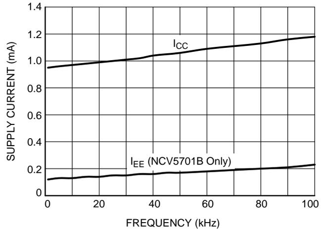
Figure 19. Supply Current vs. Switching Frequency (V<sub>CC</sub> = 15 V, V<sub>EE</sub> = -10 V, 25°C)
