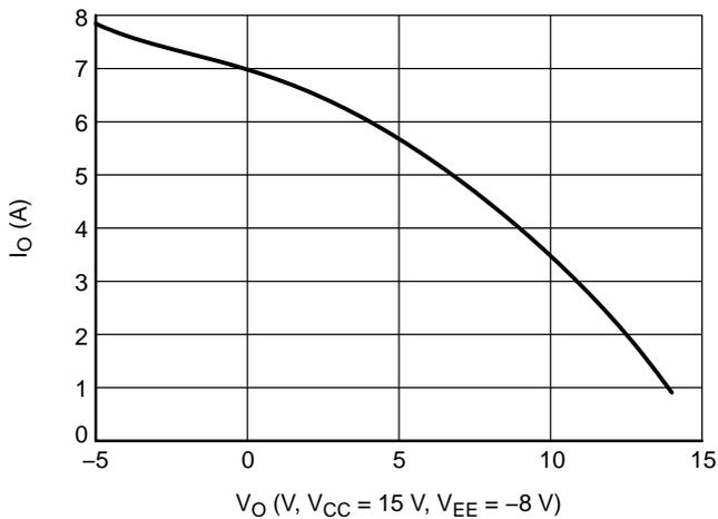
Figure 8. Output Source Current vs. Output Voltage
