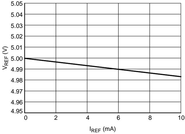
Figure 10. V<sub>REF</sub> Voltage vs. Current
