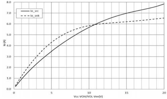
**Figure 20. Output Current vs. Output Voltage Drop**
