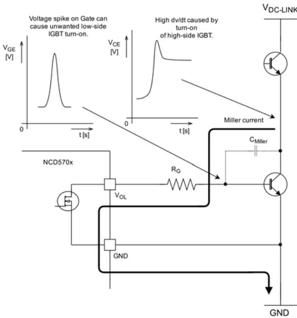
Figure 24. Current Path without Miller Clamp Protection
