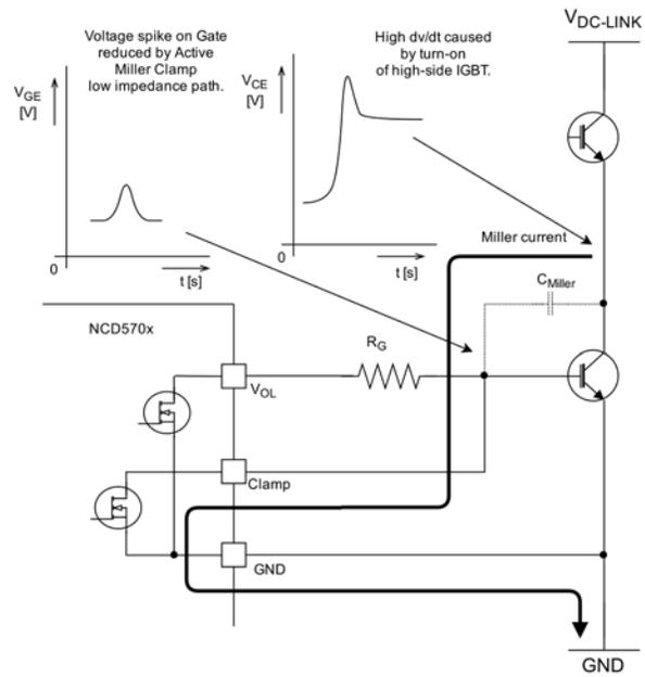
Figure 25. Current Path with Miller Clamp Protection
