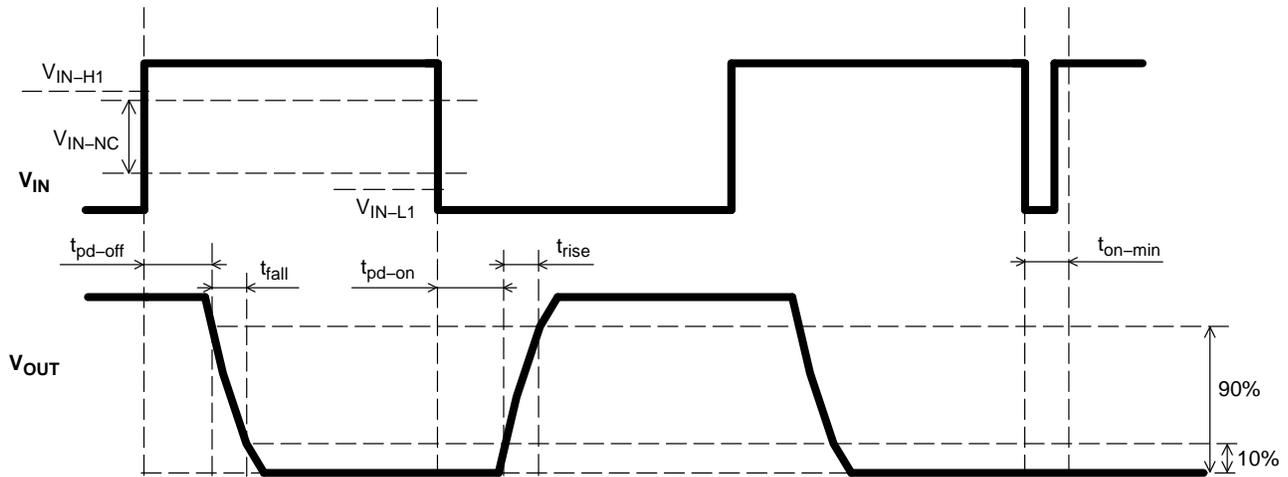
Figure 30. Input and Output Signal Parameters for Opto-coupler
