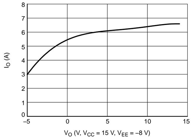
Figure 9. Output Sink Current vs. Output Voltage
