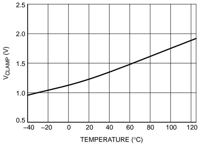
Figure 18. V<sub>CLAMP</sub> at 0.5 A (NCV5701A Only)
