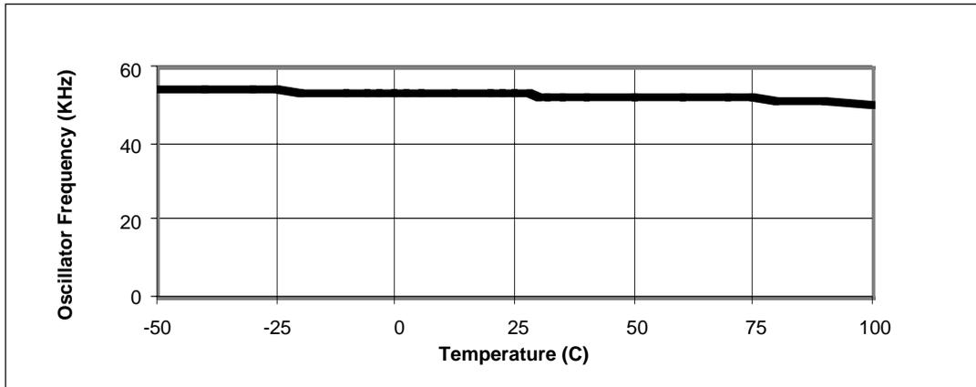
Figure 12. Oscillator Frequency vs. Temperature where FC=V+
