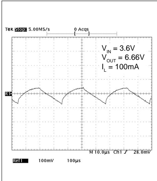
Figure 17. Output Noise and Ripple - Doubler LF
