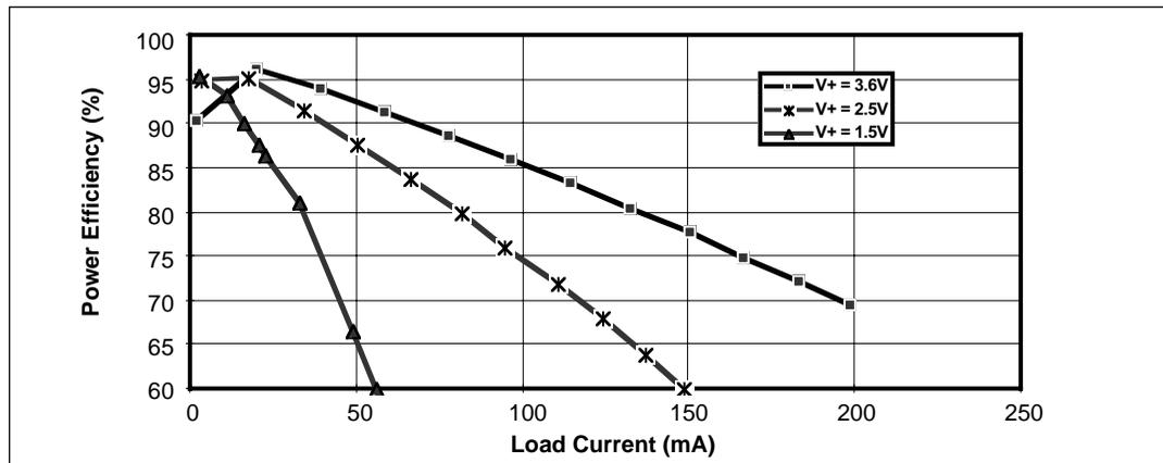
Figure 6. Power Efficiency vs. Load Current – Inverter LF
