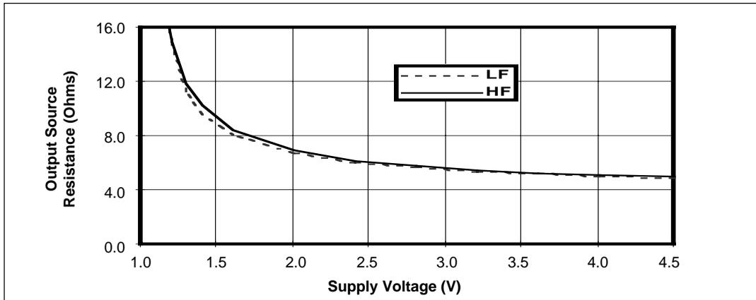
Figure 14. Output Source Resistance vs. Supply Voltage
