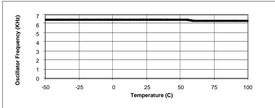
Figure 13. Oscillator Frequency vs. Temperature where FC=open
