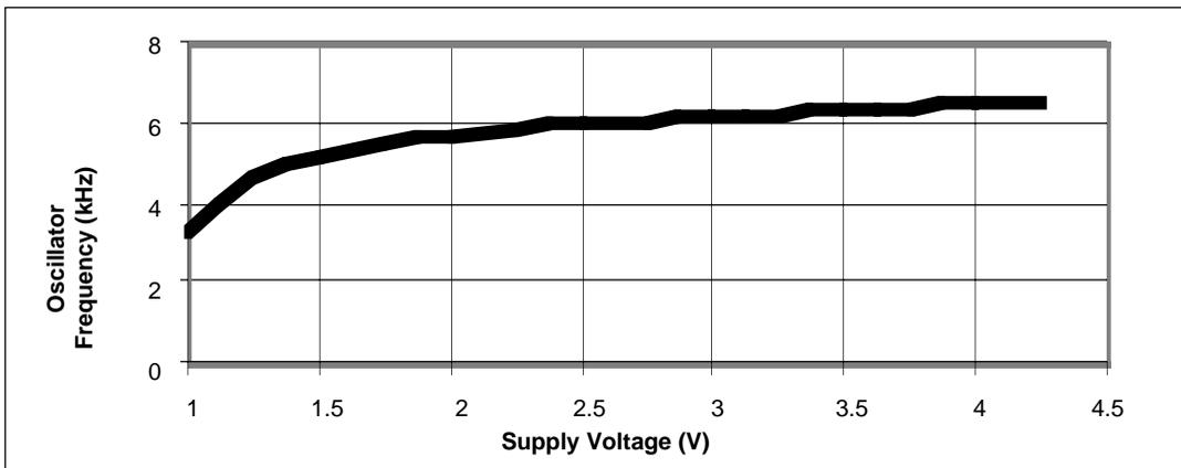
Figure 10. Oscillator Frequency vs. Supply Voltage – LF
