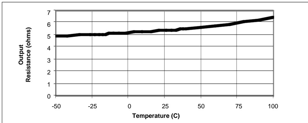
Figure 15. Output Source Resistance vs. Temperature Inverter LF
