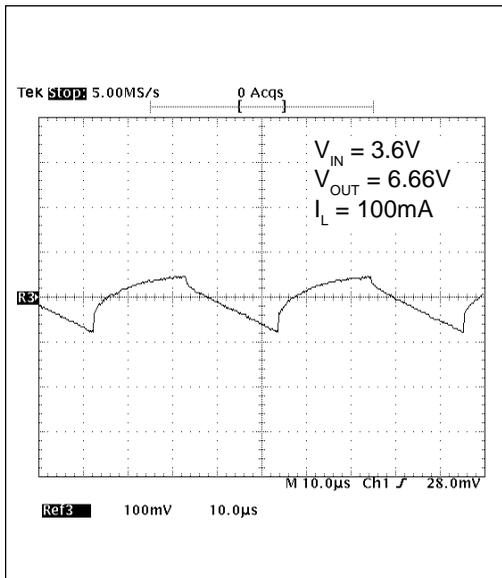
Figure 19. Output Noise and Ripple - Doubler HF
