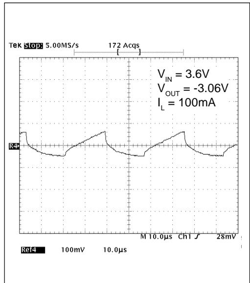
Figure 20. Output Noise and Ripple - Inverter HF
