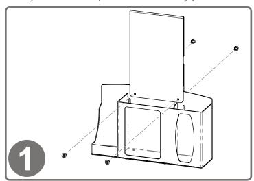
To mount the MP-070 Sign Holder, align the holes of the holder with the holes of the dispenser. With a flathead screwdriver, attach using (2x) barrel screws included with sign holder.
