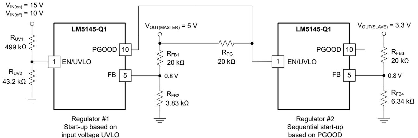
Figure 8-4. Master-Slave Sequencing Implementation Using PGOOD and EN/UVLO
