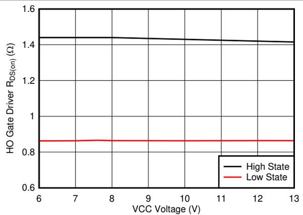
**Figure 7-22. HO Driver Resistance vs VCC Voltage**
