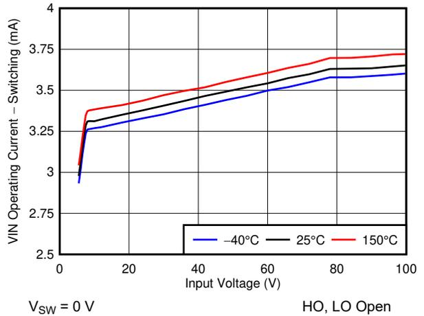
**Figure 7-8. I<sub>Q-OPERATING</sub> (Switching) vs Input Voltage**
