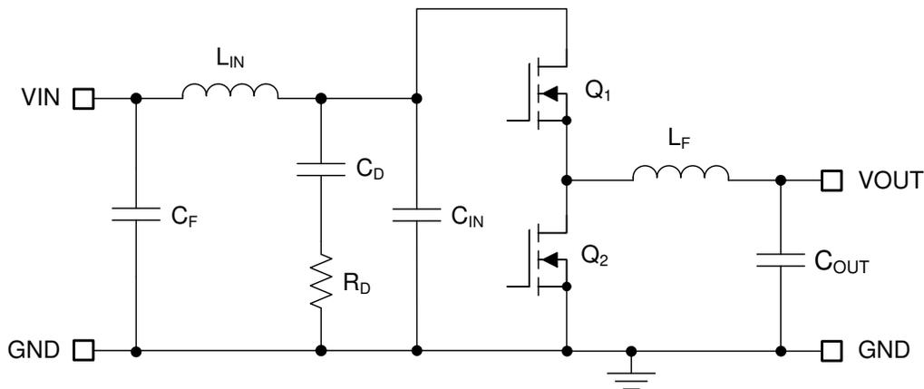
**Figure 9-4. Buck Regulator With  $\pi$ -Stage EMI Filter**
