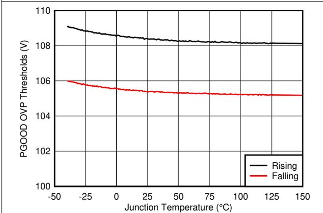
**Figure 7-15. PGOOD OVP Thresholds vs Junction Temperature**
