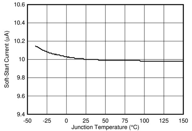
**Figure 7-28. SS/TRK Current Source vs Junction Temperature**
