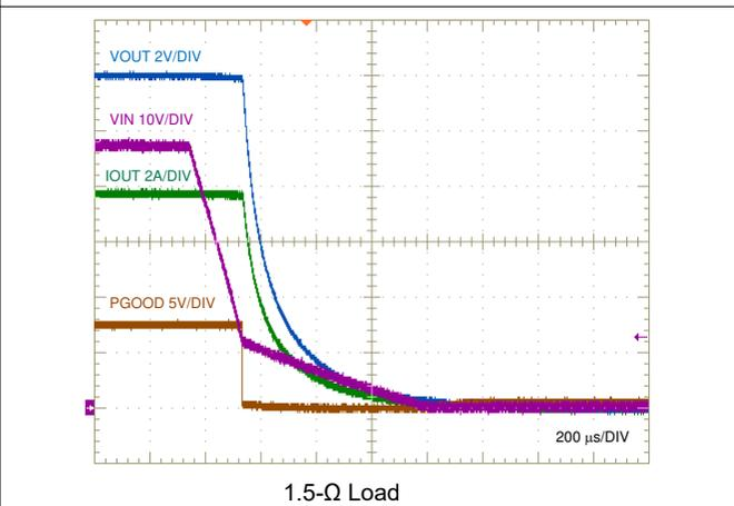
**Figure 9-20. Shutdown By Input UVLO, 8-A Resistive Load**
