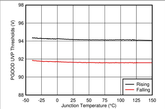
**Figure 7-14. PGOOD UVP Thresholds vs Junction Temperature**
