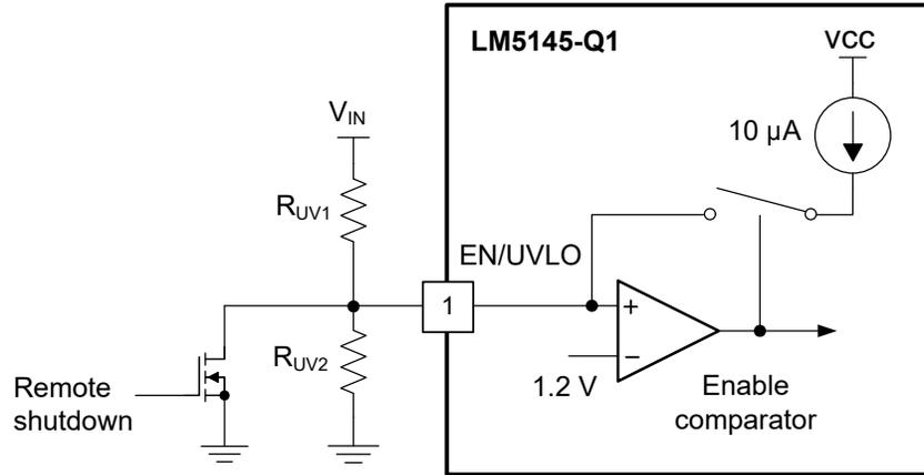
Figure 8-3. Programmable Input Voltage UVLO Turn-on and Turn-off
