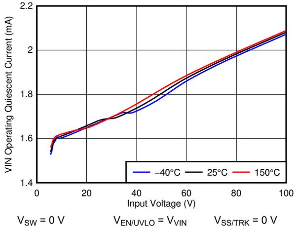
**Figure 7-7. I<sub>Q-OPERATING</sub> (Nonswitching) vs Input Voltage**
