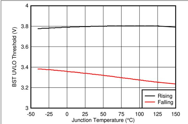
**Figure 7-13. BST UVLO Thresholds vs Junction Temperature**
