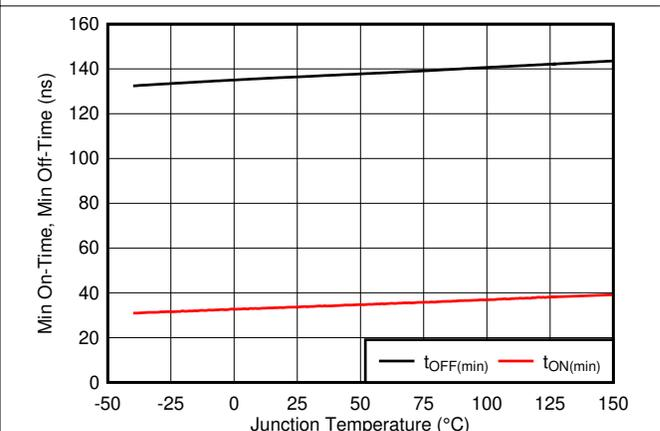
Figure 7-4.  $t_{ON(min)}$  and  $t_{OFF(min)}$  vs Junction Temperature
