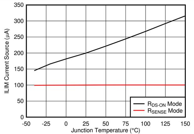
**Figure 7-10. I<sub>LIM</sub> Current Source vs Junction Temperature**
