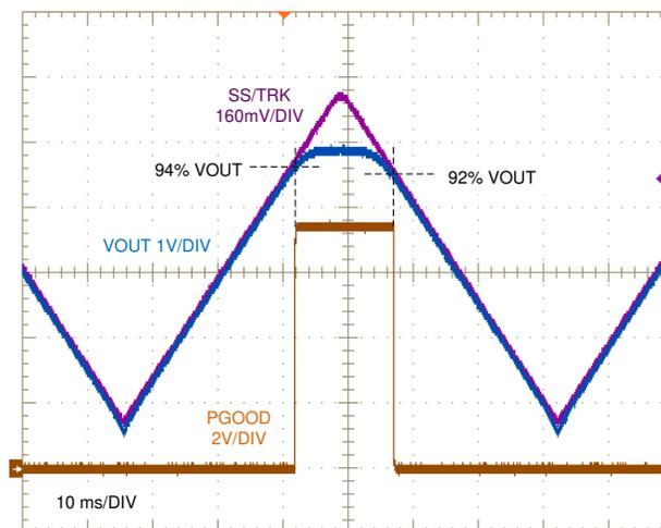
**Figure 8-6. Typical Output Voltage Tracking and PGOOD Waveforms**
