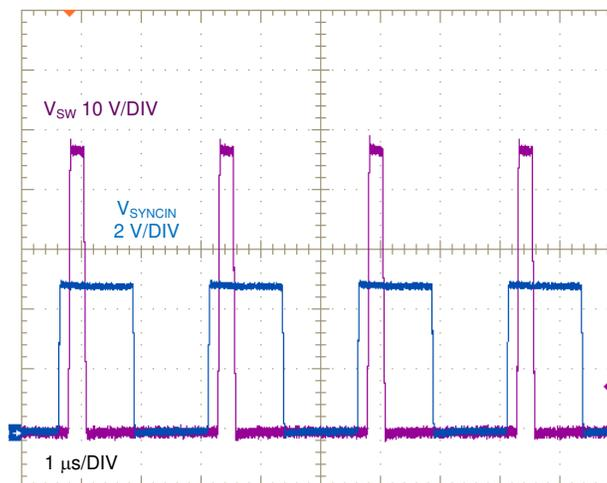
**Figure 8-5. Typical 400-kHz SYNCIN and SW Voltage Waveforms**
