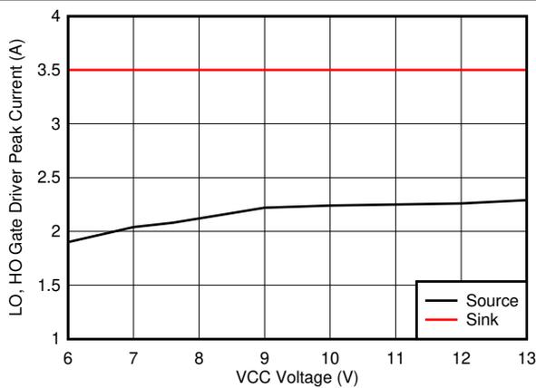
**Figure 7-21. Gate Driver Peak Current vs VCC Voltage**
