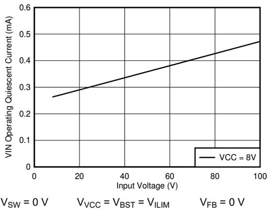
**Figure 7-9. VIN Quiescent Current with External VCC Applied**
