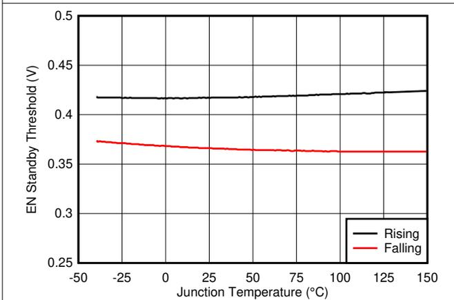
**Figure 7-17. EN Standby Thresholds vs Junction Temperature**
