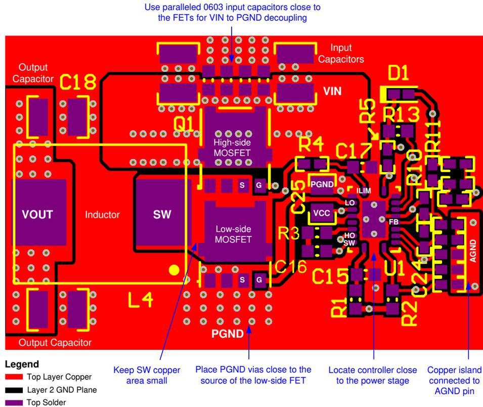
Figure 11-2. LM5145-Q1 Controller PCB Layout (Viewed From Top)
