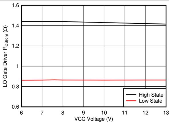
**Figure 7-23. LO Driver Resistance vs VCC Voltage**
