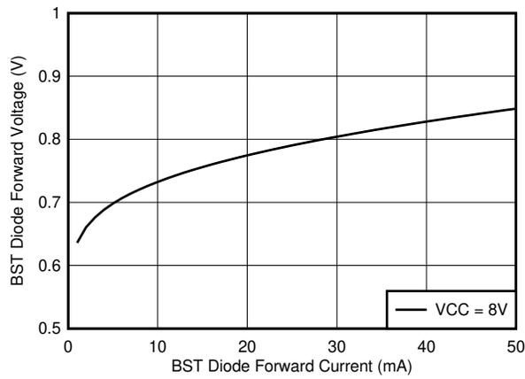
**Figure 7-27. BST Diode Forward Voltage vs Current**
