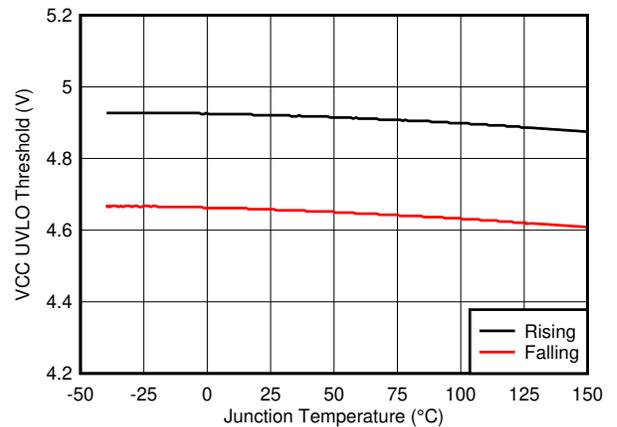
**Figure 7-12. VCC UVLO Thresholds vs Junction Temperature**
