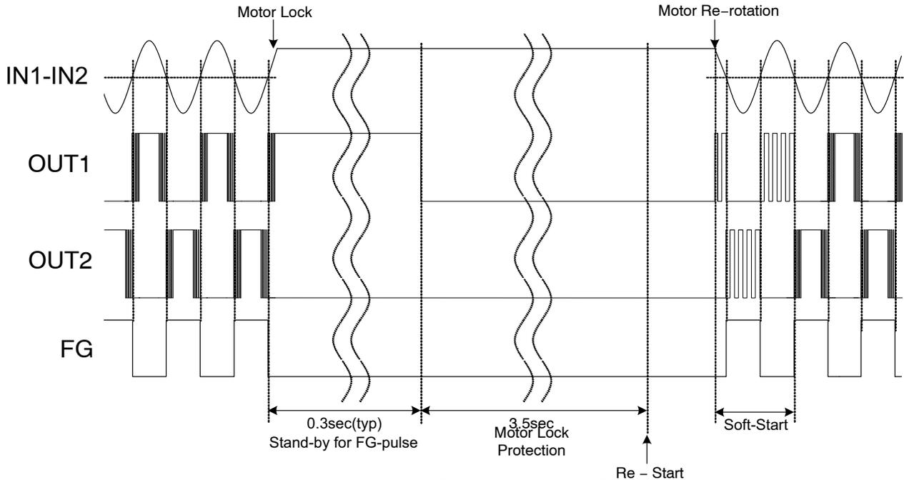
**Figure 33. Image of Lock Detection and Lock Protection**
