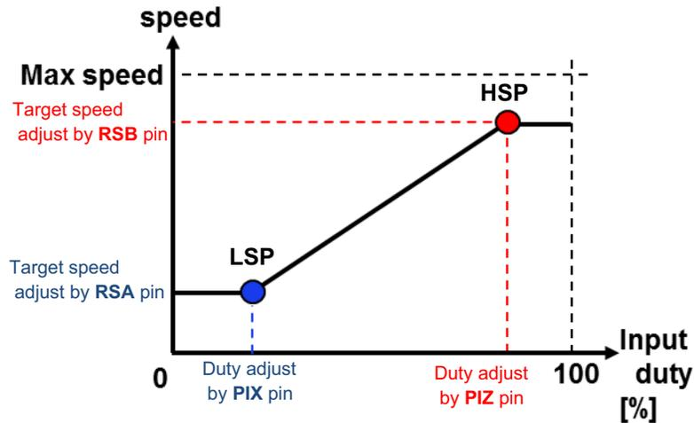
Figure 21. Speed Setting Curve Type Example 1
