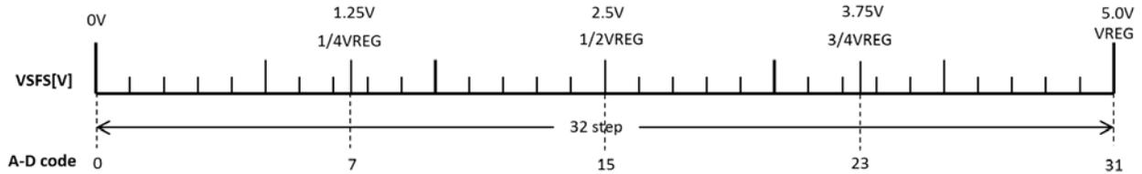
Figure 31. A-D code Figure for SFS Pin
