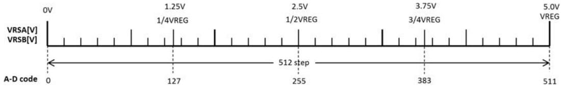
Figure 25. A-D Code Figure for RSA/RSB Pin
