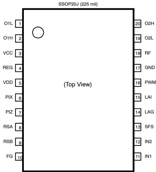
Figure 3. LV88551JA, LV88552JA, LV88553JA, LV88554JA Pin Assignment
