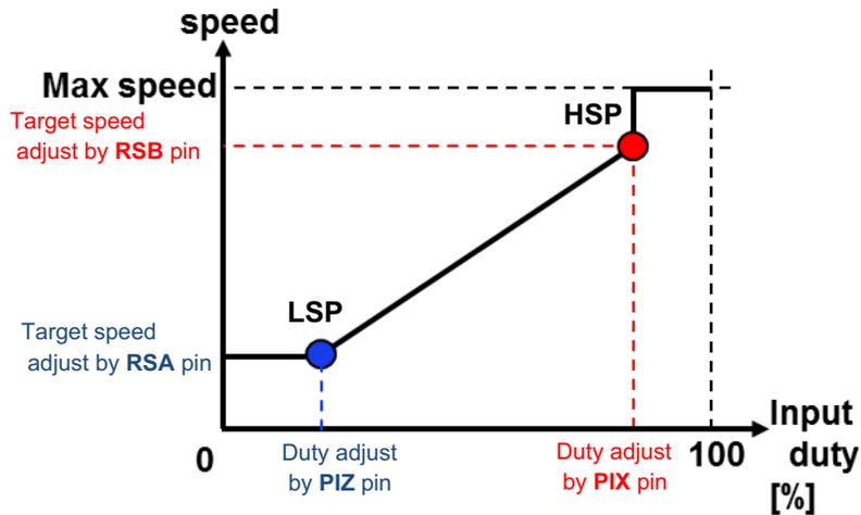
Figure 24. Speed Setting Curve Type Example 4
