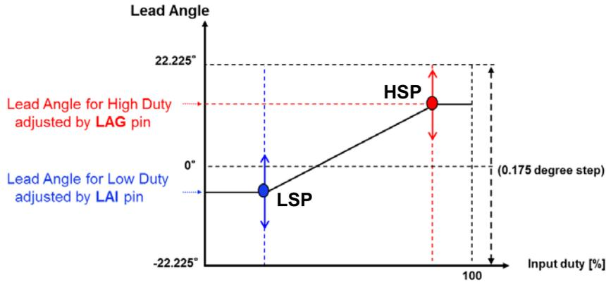
Figure 28. Image of Lead Angle Setting Curve
