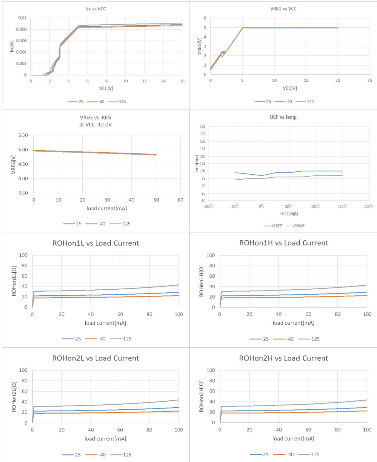
Figure 6. Typical Characteristics
