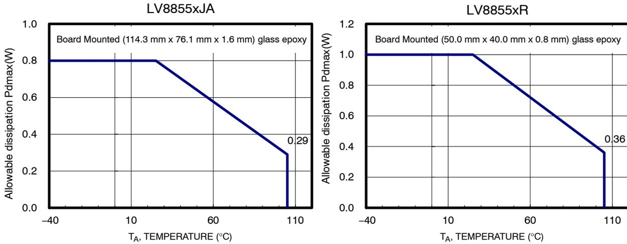
**Figure 5. Power Dissipation vs Ambient Temperature Characteristic**
