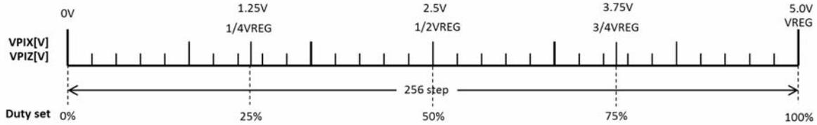
Figure 26. Input Duty Parameter Setting for PIX/PIZ Pin
