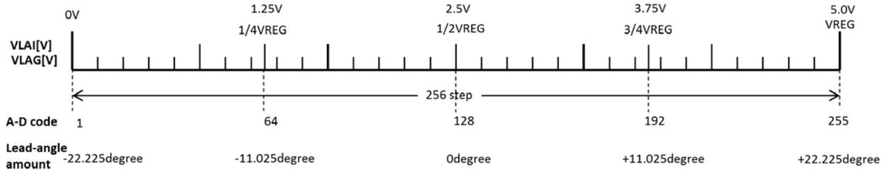
Figure 27. Lead-Angle Parameter Setting for LAI/LAG Pin
