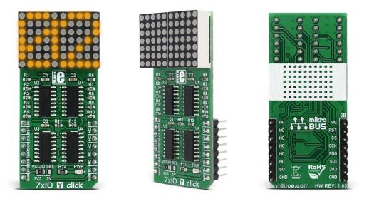
**7x10 Y click** displays letters, numbers, and characters in a 7x5 font resolution. It carries a matrix of 70 yellow LEDs driven by a pair of 8-bit serial-in, parallel-out shift registers, a Darlington Transistor array and a Johnson counter.
