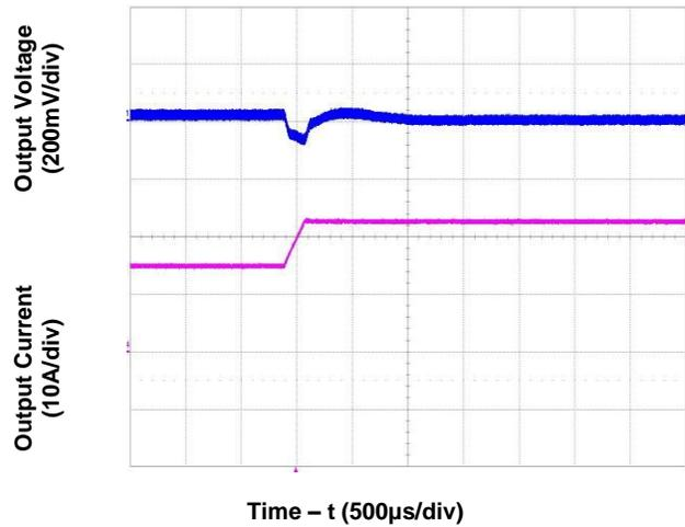
**Figure 8. Transient Load Response**
