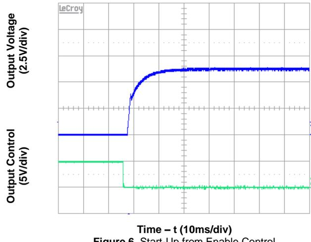
Figure 6. Start-Up from Enable Control (typical Vin, zero load, external Cap.=1000µF)
