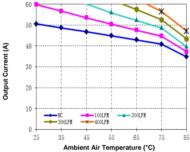
**Figure 9. Current Derating Curve for Airflow Direction 3**
