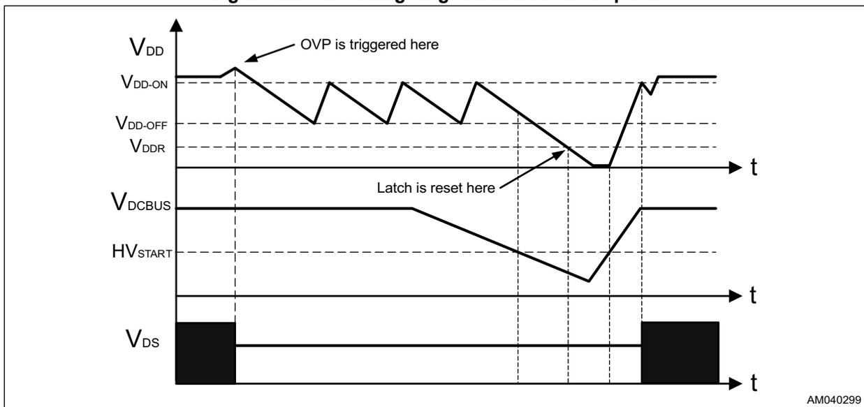
Figure 13. OVP function: timing diagram
