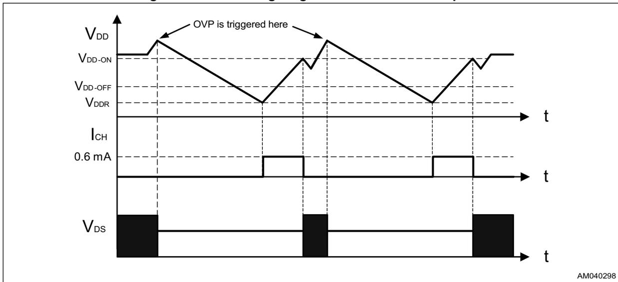
**Figure 12. OVP timing diagram with latched option**
