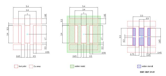
For superior solder joint connectivity results we recommend soldering under standard nitrogen atmosphere. Further information can be found in our Application Note: "Handling and Processing Details for Ceramic LEDs". Package not suitable for any kind of wet cleaning or ultrasonic cleaning.
