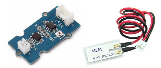
Grove-Piezo Vibration Sensor is suitable for measurements of flexibility, vibration, impact and touch. The module is based on PZT film sensor LDT0-028. When the sensor moves back and forth, a certain voltage will be generated by the voltage comparator inside of it. A wide dynamic range (0.001Hz~1000MHz) guarantees an excellent measuring performance. And, you can adjust its sensitivity by adjusting the on-board potentiometer with a screw.
