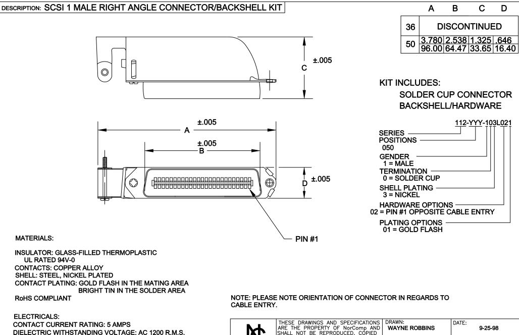
INSULATION RESISTANCE: 1000 mohms MINIMUM AT 500V DC
