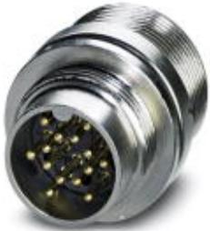
Device connector, front mounting, straight, Screw locking, M16, Number of positions: 8, Type of contact: Male connector, Solder connection, Axial O-ring, Central fixing, Shielded: No
