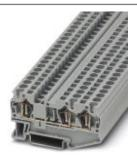
Feed-through terminal block, Connection method: Spring-cage connection, Cross section: 0.08 mm² - 6 mm², AWG: 28 - 10, Width: 6.2 mm, Color: brown, Mounting type: NS 35/7,5, NS 35/15
