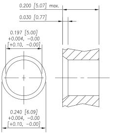
RECOMMEND PANEL CUT-OUT MAX. PANEL THICKNESS: 0.200" [5.08]
