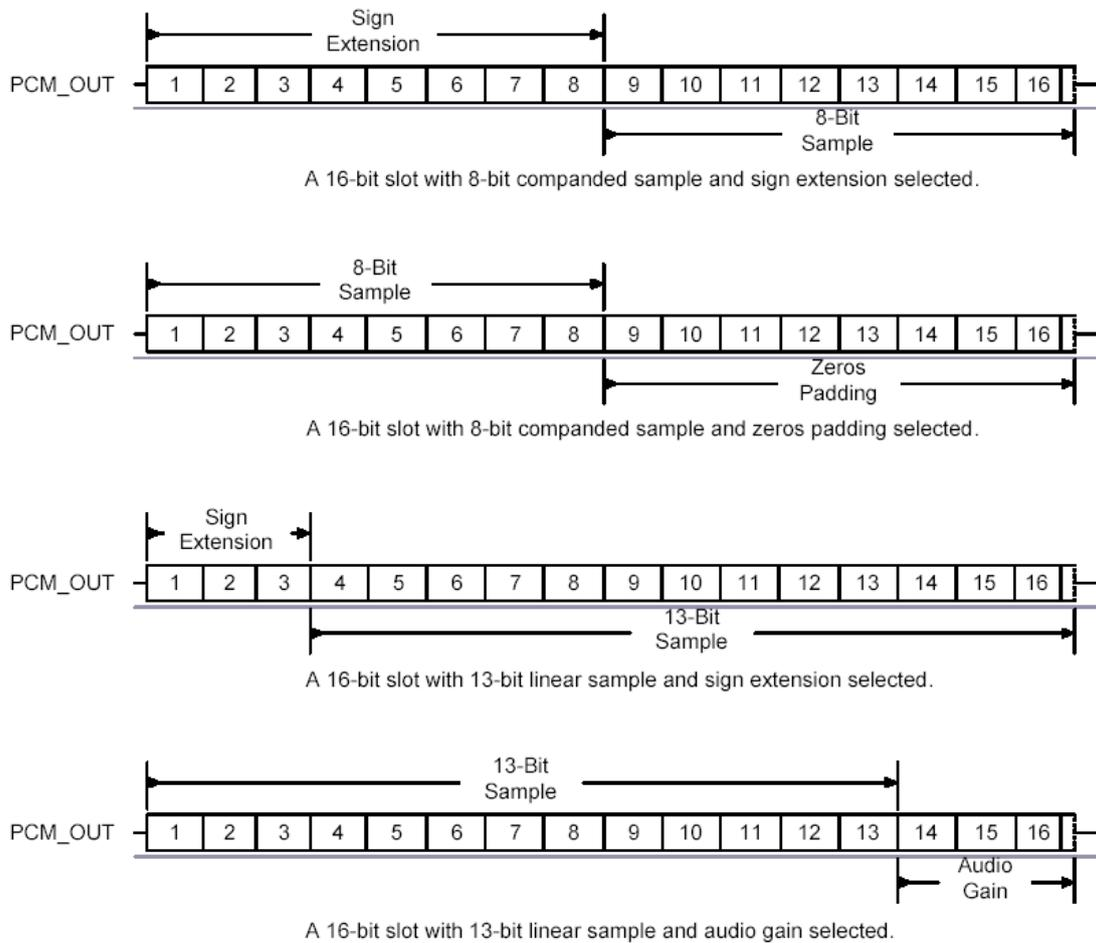
**Figure 31: 16-bit Slot Length and Sample Formats**
