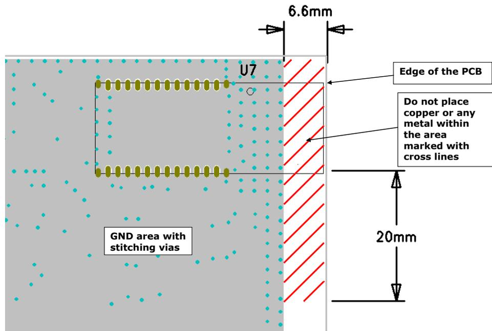
Figure 15: Recommended metal keep put area for WT11u
