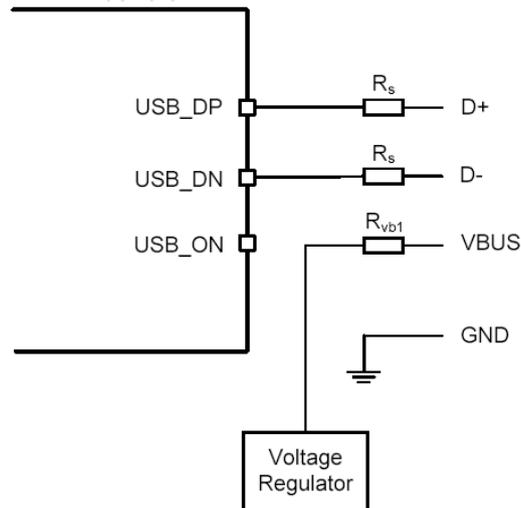
**Figure 23: USB Connections for Bus-Powered Mode**
