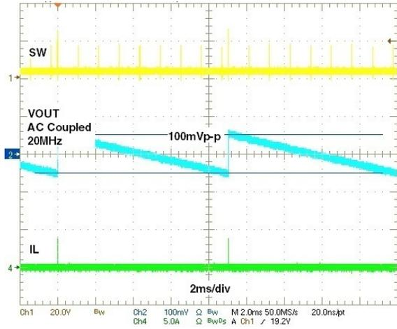
Figure 14: Steady state, DCM,  $I_{OUT} = 0A$
