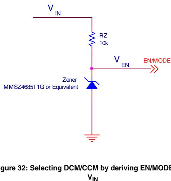
Figure 32: Selecting DCM/CCM by deriving EN/MODE from  $V_{IN}$
