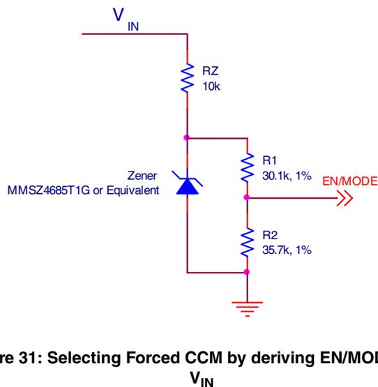
Figure 31: Selecting Forced CCM by deriving EN/MODE from  $V_{IN}$
