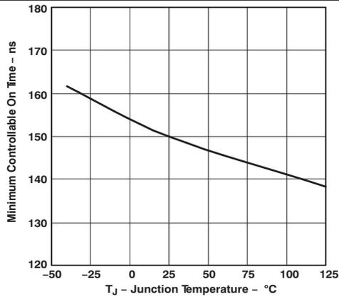
**Figure 7. Minimum Controllable On Time vs. Junction Temperature**
