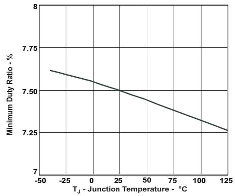
**Figure 8. Minimum Controllable Duty Ratio vs. Junction Temperature**
