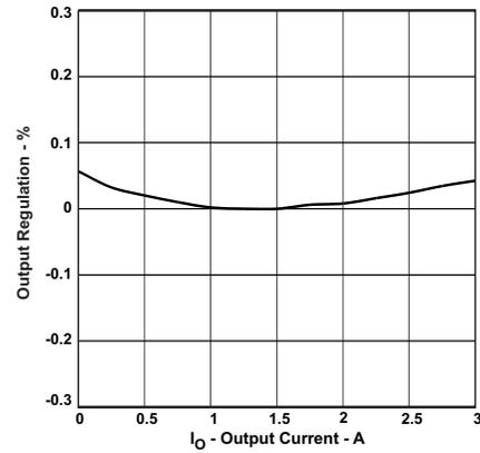
Figure 11. Output Regulation % vs. Output Current
