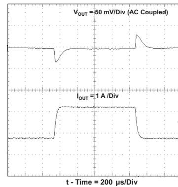
Figure 15. Transient Response,  $I_O$  Step 0.75 to 2.25 A.
