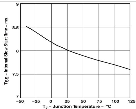
Figure 6. Internal Slow Start Time vs. Junction Temperature
