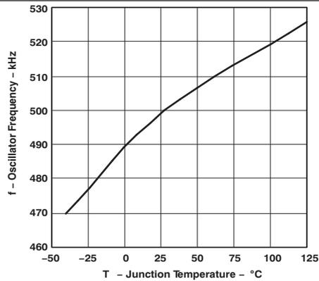
Figure 1. Oscillator Frequency vs. Junction Temperature
