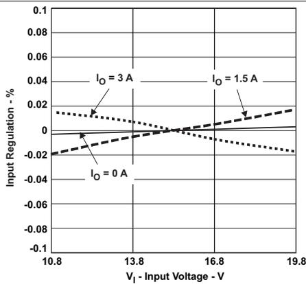
Figure 12. Input Regulation % vs. Input Voltage
