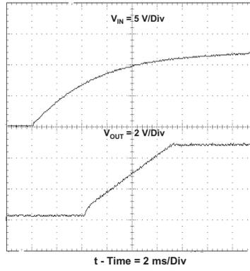
Figure 16. Startup Waveform,  $V_{IN}$  and  $V_{OUT}$ .
