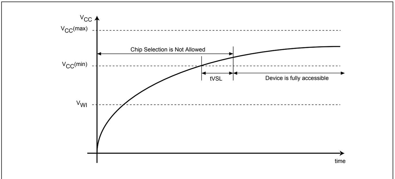
**Figure 137. Power Up/Down and Voltage Drop**
