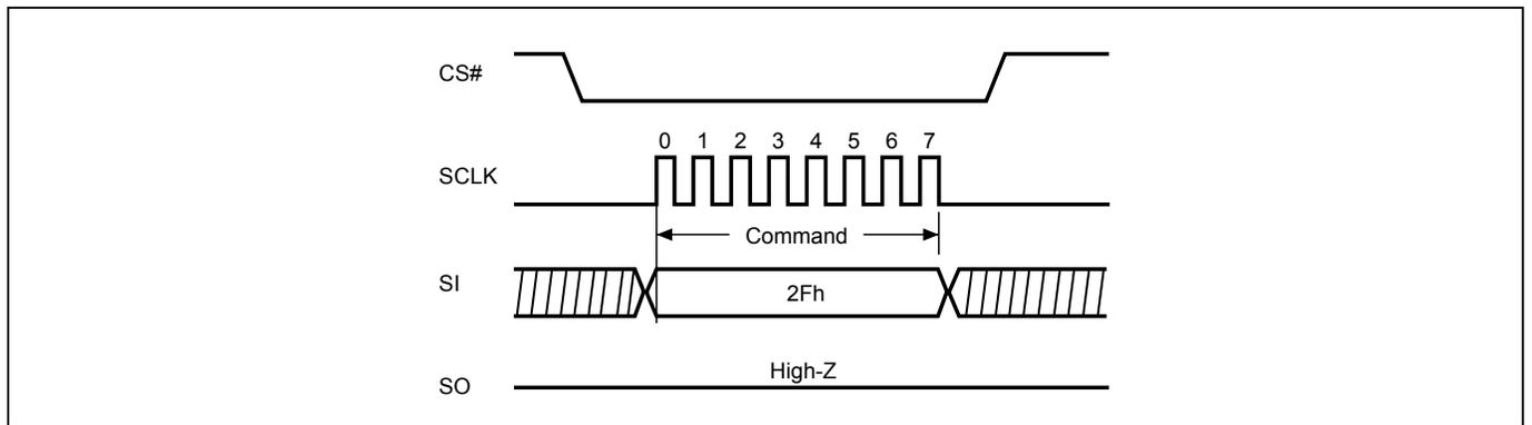
**Figure 38. Write Security Register (WRSCUR) Sequence (STR-OPI Mode)**
