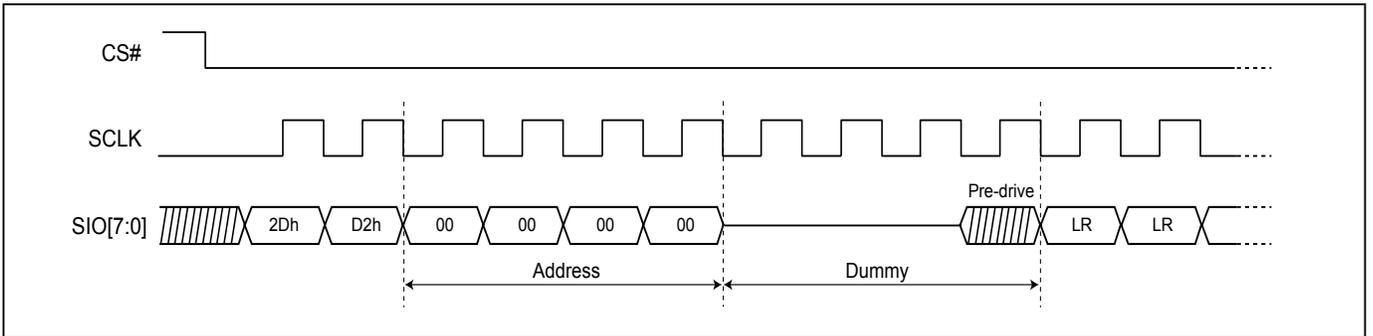
**Figure 82. Read Lock Register (RDLR) Sequence (DTR-OPI Mode)**
