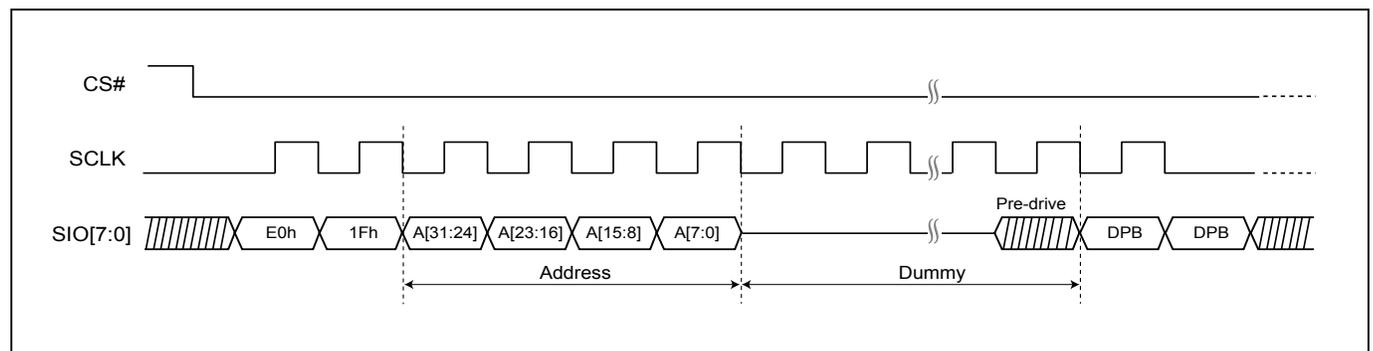
**Figure 99. Read DPB Register (RDDPB) Sequence (DTR-OPI Mode)**
