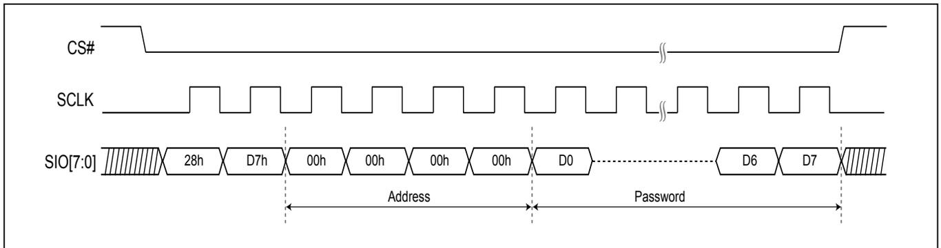
**Figure 106. Write Password Register (WRPASS) Sequence (DTR-OPI Mode)**
