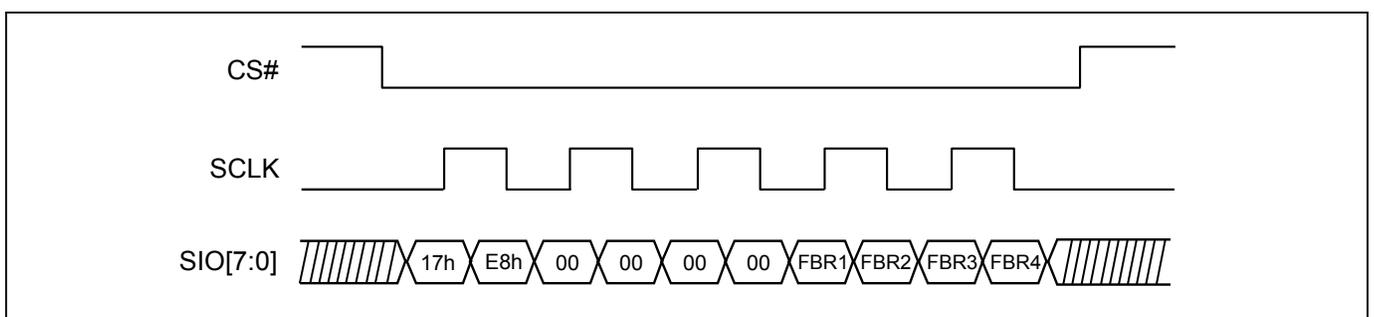
**Figure 58. Erase Fast Boot Register (ESFBR) Sequence**
