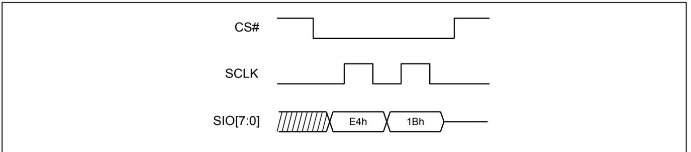
**Figure 91. SPB Erase (ESSPB) Sequence (DTR-OPI Mode)**
