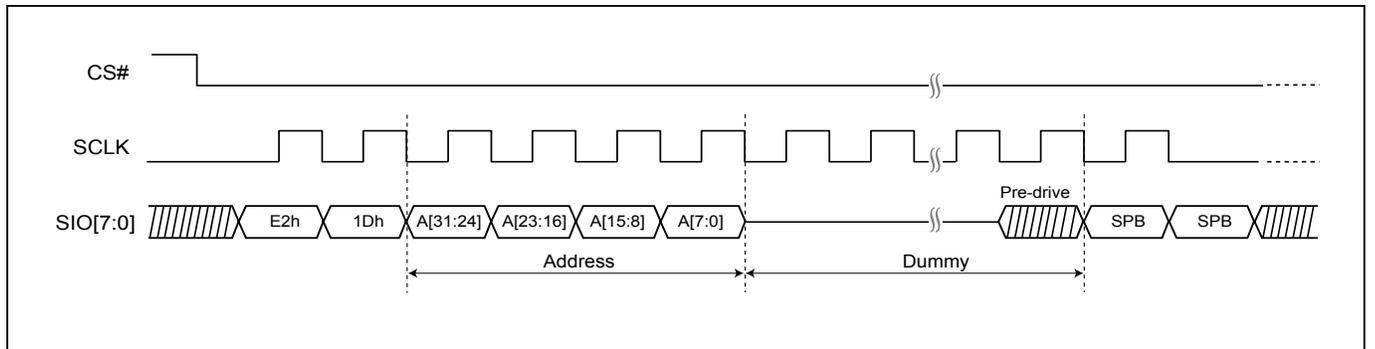
**Figure 88. Read SPB Status (RDSPB) Sequence (DTR-OPI Mode)**
