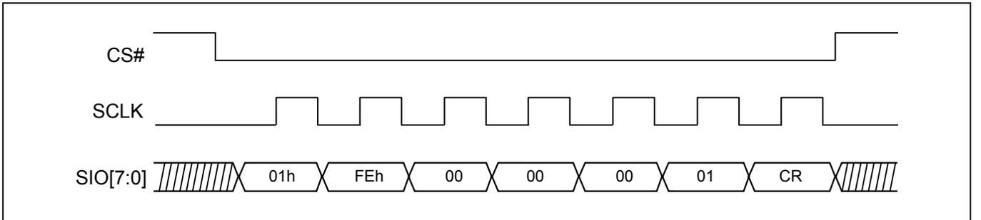
**Figure 26. Write Configuration Register (WRCR) Sequence (DTR-OPI Mode)**
