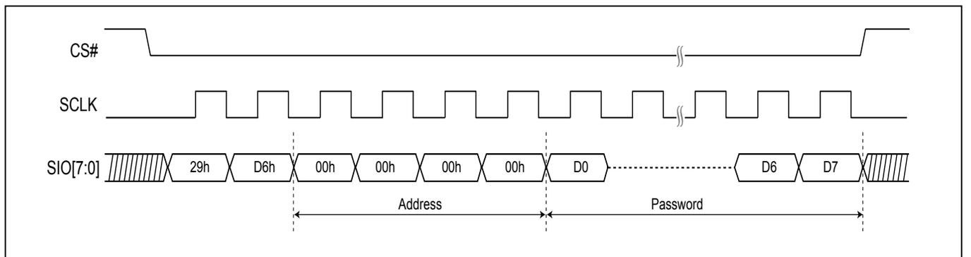
**Figure 109. Password Unlock (PASSULK) (DTR-OPI Mode)**
