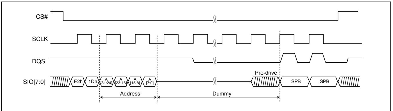
**Figure 89. SPB Erase (ESSPB) Sequence**
