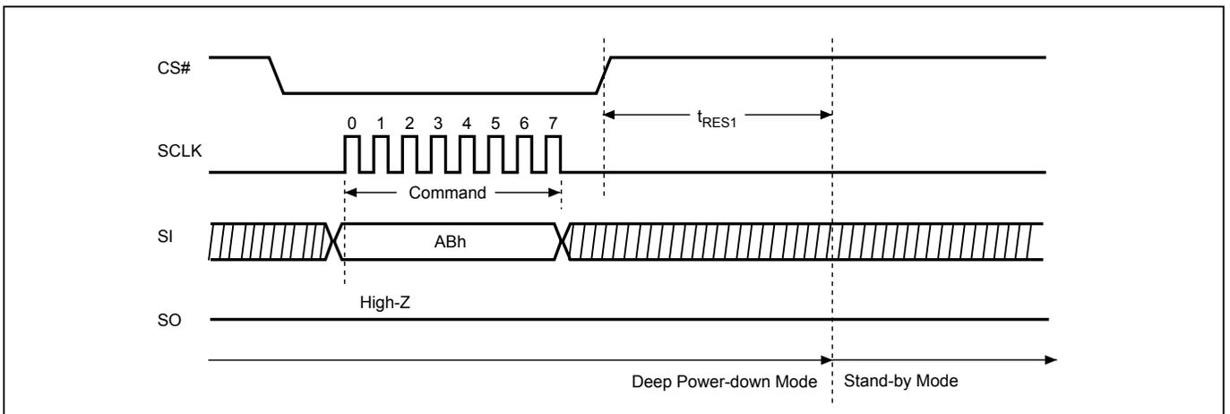
**Figure 77. Release from Deep Power-down (RDP) Sequence (STR-OPI Mode)**
