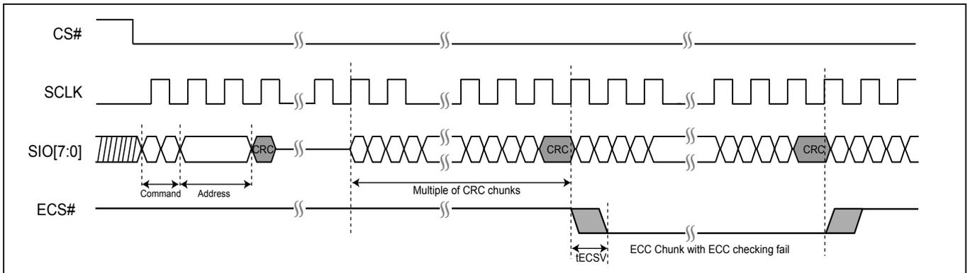
**Figure 122. CRC Timing (With CRC# output)**
