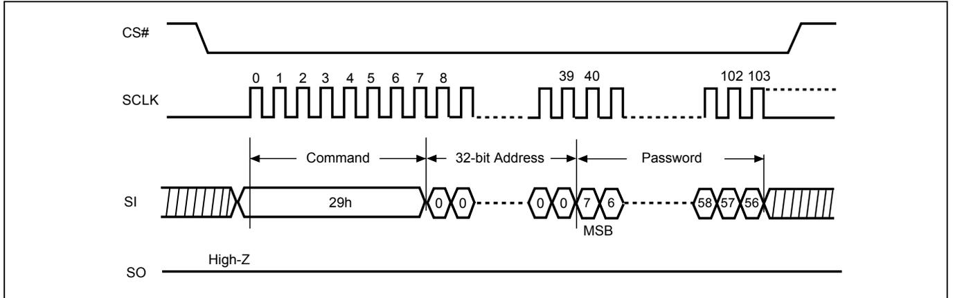
**Figure 108. Password Unlock (PASSULK) (STR-OPI Mode)**
