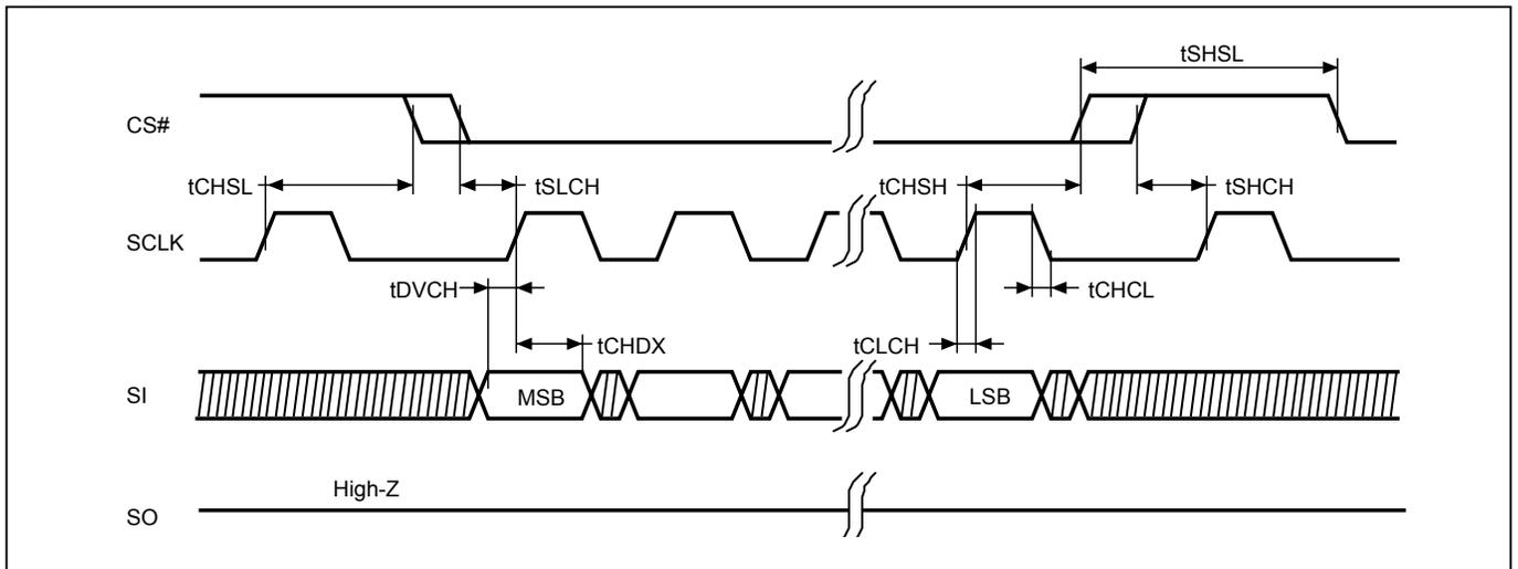
**Figure 2. Input Timing (DTR mode)**
