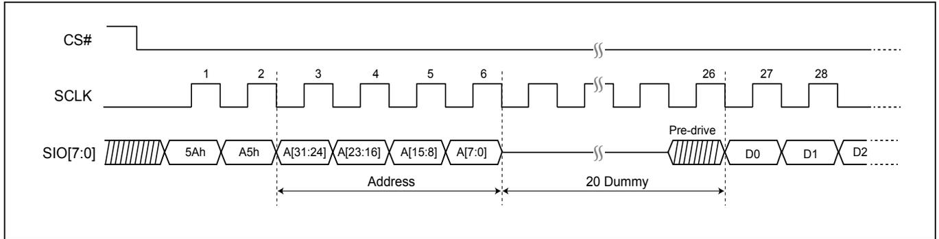
**Figure 119. Read Serial Flash Discoverable Parameter (RDSFDP) Sequence (DTR-OPI Mode)**
