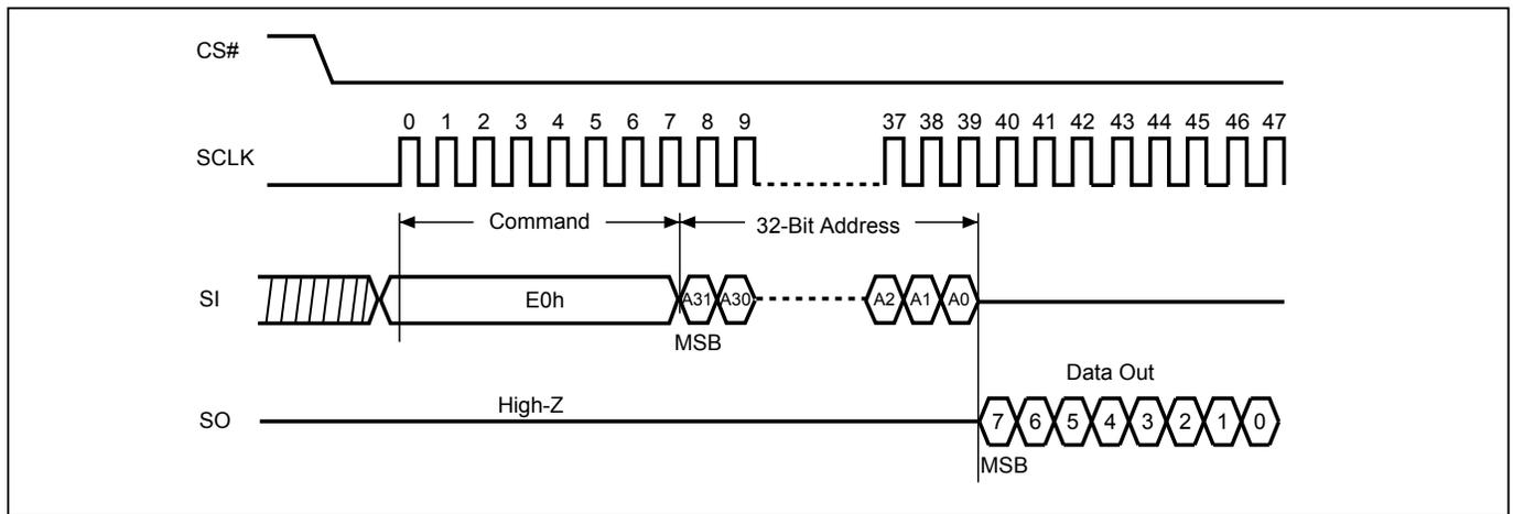
**Figure 96. Read DPB Register (RDDPB) Sequence (STR-OPI Mode)**
