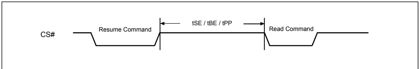
**Figure 112. Resume to Suspend Latency**
