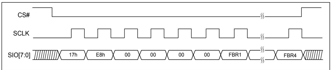
**Figure 57. Write Fast Boot Register (WRFBR) Sequence (DTR-OPI Mode)**
