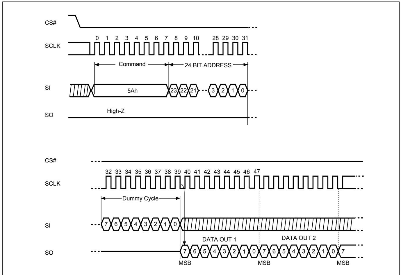
**Figure 118. Read Serial Flash Discoverable Parameter (RDSFDP) Sequence (STR-OPI Mode)**
