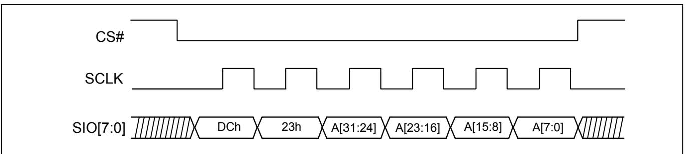
**Figure 66. Block Erase (BE) Sequence (DTR-OPI Mode)**
