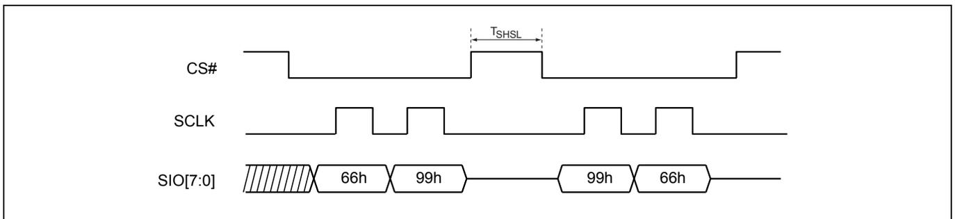
**Figure 116. Reset Sequence (DTR-OPI mode)**
