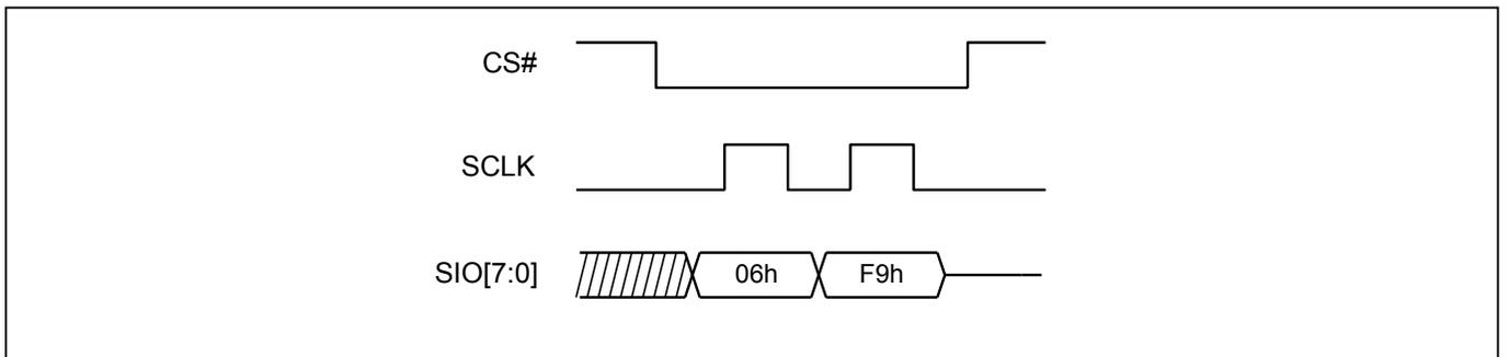
**Figure 7. Write Enable (WREN) Sequence (DTR-OPI Mode)**
