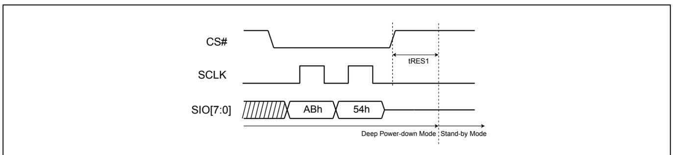
**Figure 78. Release from Deep Power-down (RDP) Sequence (DTR-OPI Mode)**
