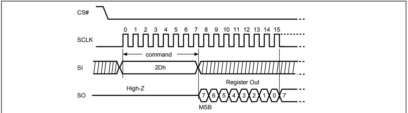
**Figure 81. Read Lock Register (RDLR) Sequence (STR-OPI Mode)**
