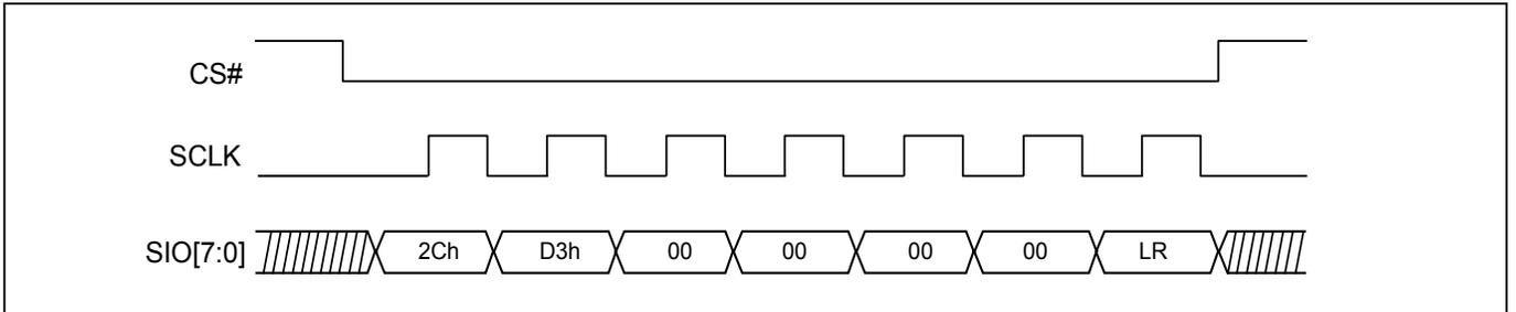
**Figure 85. Write Lock Register (WRLR) Sequence (DTR-OPI Mode)**
