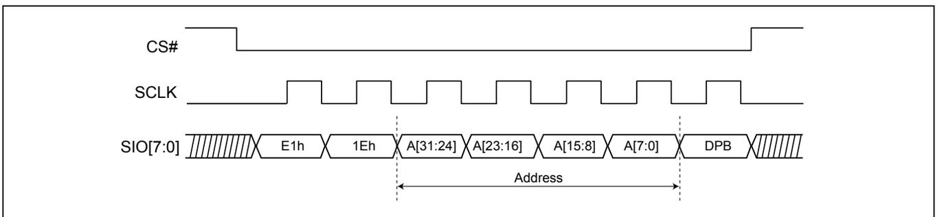
**Figure 100. Write DPB Register (WRDPB) Sequence (DTR-OPI Mode)**
