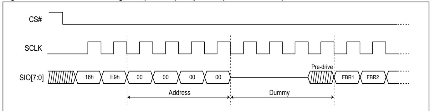
**Figure 54. Read Fast Boot Register (RDFBR) Sequence (DTR-OPI Mode)**
