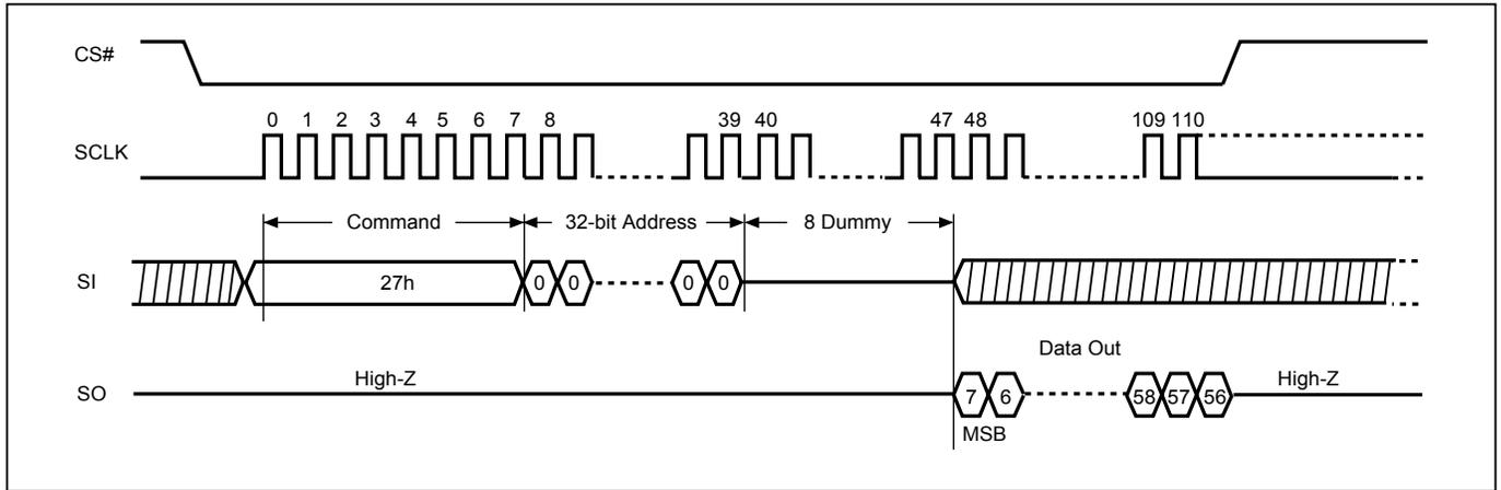
**Figure 102. Read Password Register (RDPASS) Sequence (STR-OPI Mode)**
