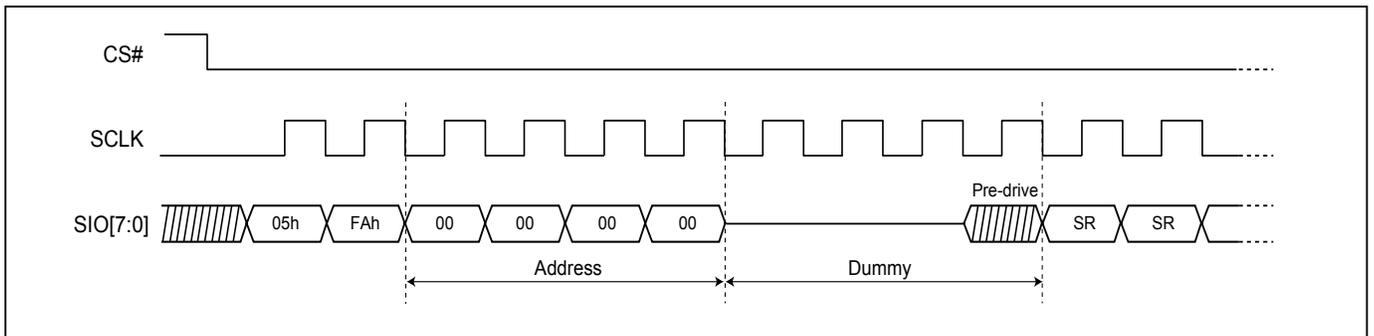
**Figure 16. Read Status Register (RDSR) Sequence (DTR-OPI Mode)**
