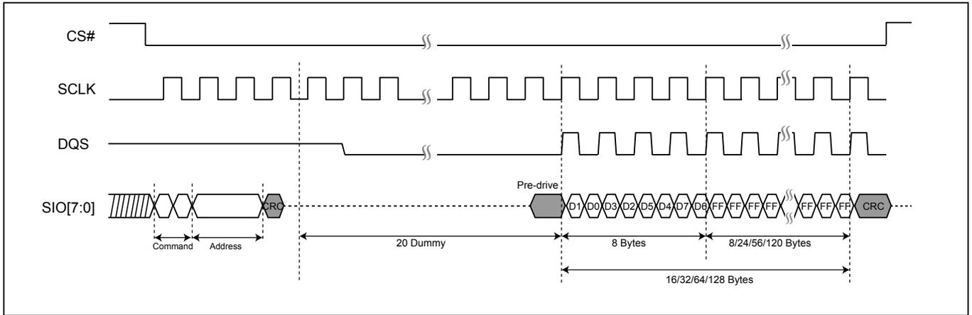
**Figure 127. CRC Timing (WRPASS/PASSULK)**
