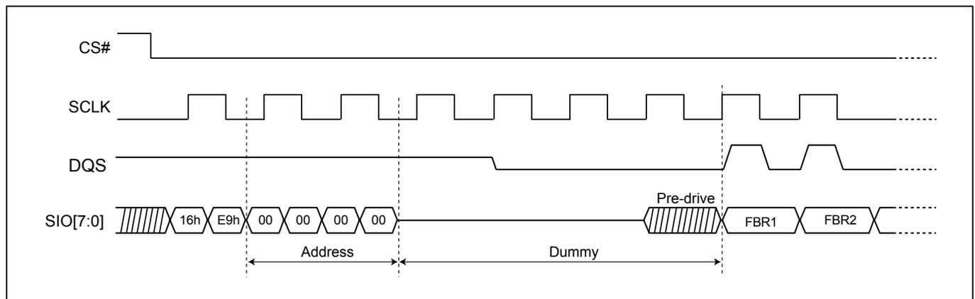
**Figure 55. Write Fast Boot Register (WRFBR) Sequence**
