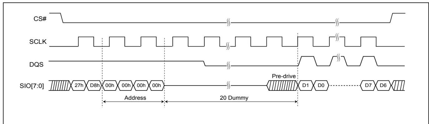
**Figure 104. Write Password Register (WRPASS) Sequence**
