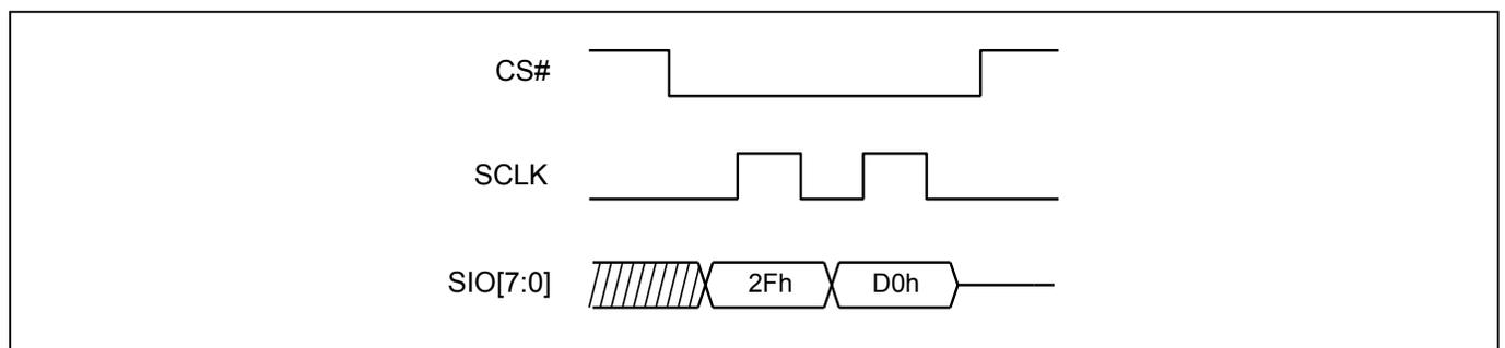
**Figure 39. Write Security Register (WRSCUR) Sequence (DTR-OPI Mode)**
