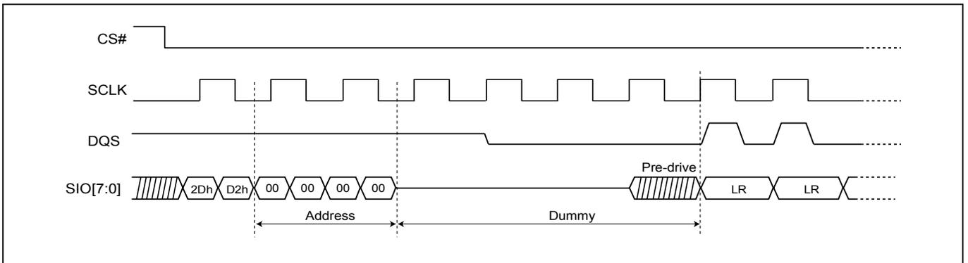
**Figure 83. Write Lock Register (WRLR) Sequence**
