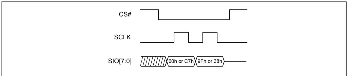
**Figure 69. Chip Erase (CE) Sequence (DTR-OPI Mode)**
