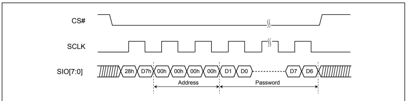
**Figure 107. Password Unlock (PASSULK) Sequence**
