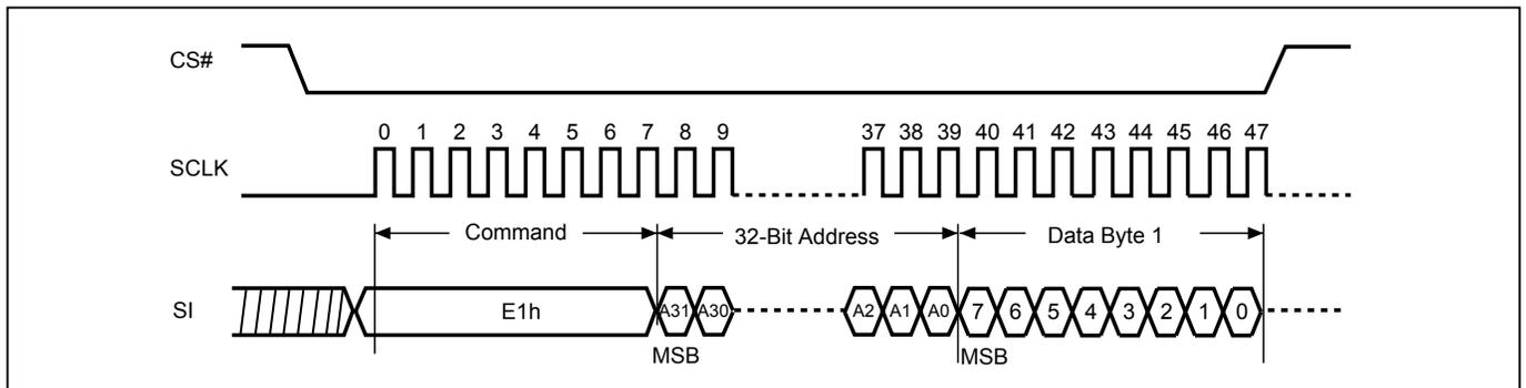
**Figure 98. Write DPB Register (WRDPB) Sequence (STR-OPI Mode)**
