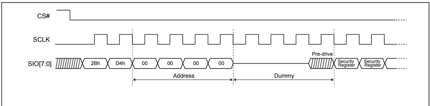
**Figure 36. Read Security Register (RDSCUR) Sequence (DTR-OPI Mode)**
