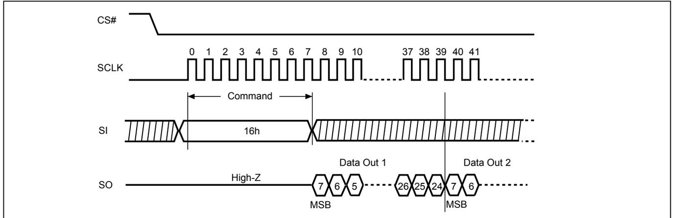
**Figure 53. Read Fast Boot Register (RDFBR) Sequence (STR-OPI Mode)**
