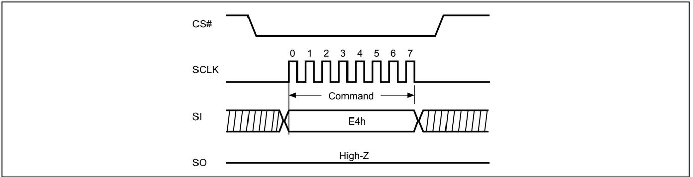
**Figure 90. SPB Erase (ESSPB) Sequence (STR-OPI Mode)**
