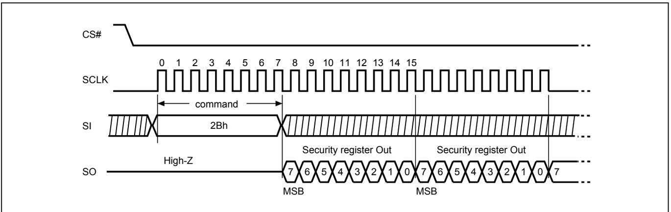
**Figure 35. Read Security Register (RDSCUR) Sequence (STR-OPI Mode)**
