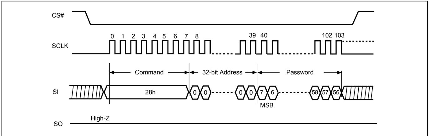
**Figure 105. Write Password Register (WRPASS) Sequence (STR-OPI Mode)**
