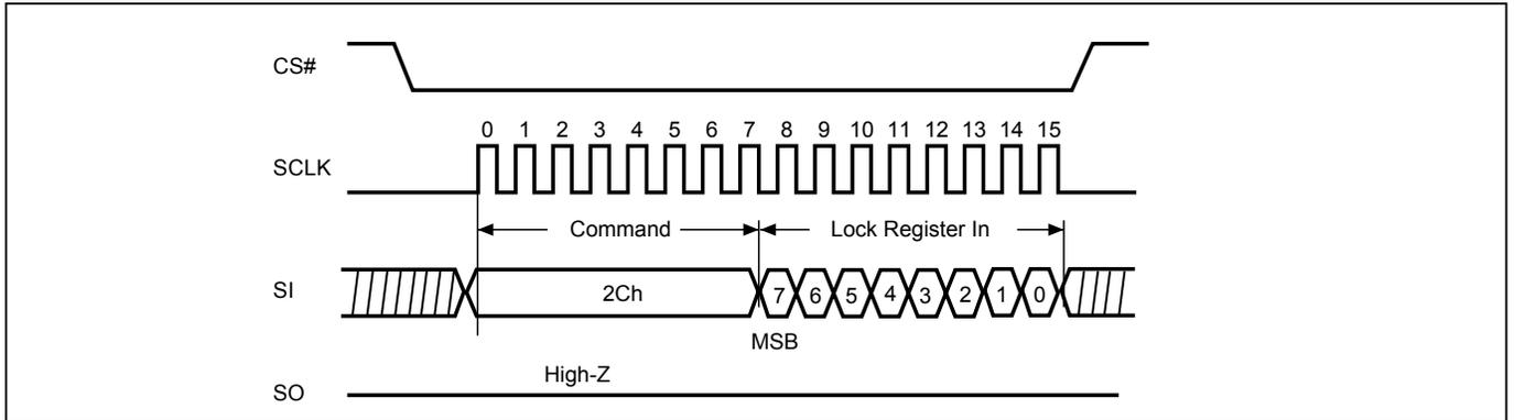
**Figure 84. Write Lock Register (WRLR) Sequence (STR-OPI Mode)**
