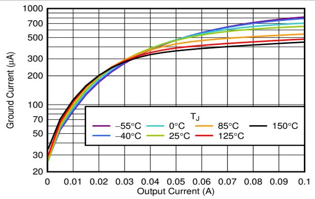
**Figure 6-6.  $I_{GND}$  vs  $I_{OUT}$  ( $MID\_OUT$  in Dropout)**
