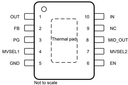
**Figure 5-1. DGQ Package (Adjustable), 10-Pin HVSSOP (Top View)**
