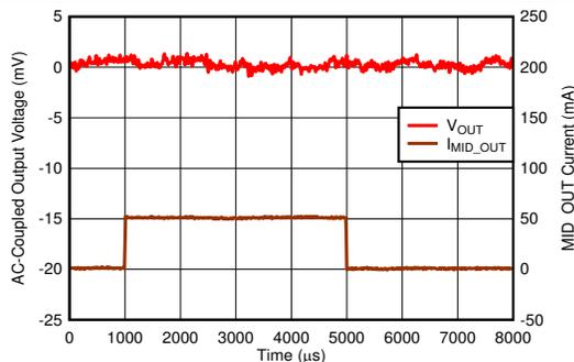
$V_{IN} = 65\text{ V}$ ,  $V_{OUT} = 3.3\text{ V}$ ,  $I_{MID\_OUT} = 0\text{ mA}$  to  $50\text{ mA}$  to  $0\text{ mA}$ ,
