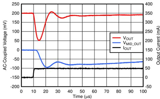
$V_{IN} = 65\text{ V}$ ,  $V_{OUT} = 3.3\text{ V}$ ,  $I_{OUT} = 1\text{ mA}$  to  $50\text{ mA}$  to  $1\text{ mA}$ ,
