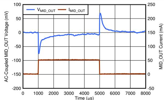
$V_{IN} = 65\text{ V}$ ,  $V_{MID\_OUT} = 12\text{ V}$ ,  $I_{MID\_OUT} = 1\text{ mA}$  to  $50\text{ mA}$  to  $1\text{ mA}$ ,
