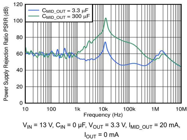
**Figure 6-37. MID\_OUT PSRR vs Frequency and  $C_{\text{MID\_OUT}}$**
