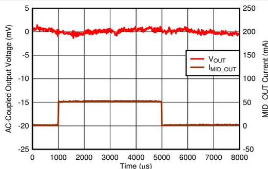
$V_{IN} = 65\text{ V}$ ,  $V_{OUT} = 3.3\text{ V}$ ,  $I_{MID\_OUT} = 1\text{ mA}$  to  $50\text{ mA}$  to  $1\text{ mA}$ ,
