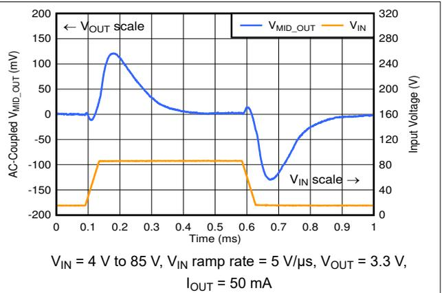
Figure 6-20. Line Transient ( $V_{MID\_OUT}$  in Dropout)
