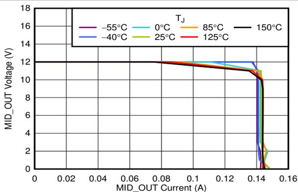
**Figure 6-5.  $V_{MID\_OUT}$  vs  $I_{MID\_OUT}$**
