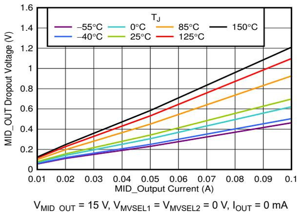
Figure 6-11.  $V_{DO(MID\_OUT)}$  vs  $I_{MID\_OUT}$
