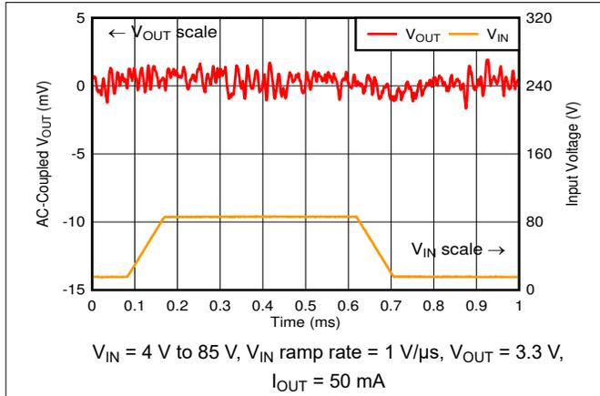
Figure 6-19. Line Transient ( $V_{MID\_OUT}$  in Dropout)
