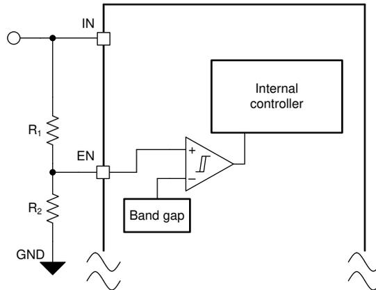
**Figure 7-3. Enable the Device Using the Input Voltage**
