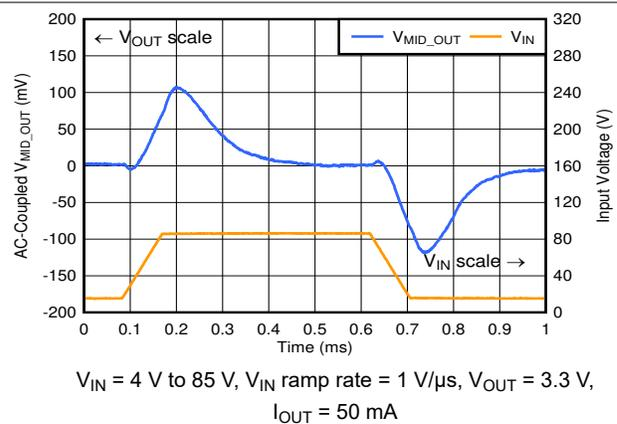
**Figure 6-18. Line Transient ( $V_{MID\_OUT}$  in Dropout)**
