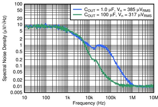
$V_{IN} = 13\text{ V}$ ,  $V_{OUT} = 3.3\text{ V}$ ,  $I_{OUT} = 20\text{ mA}$ ,
