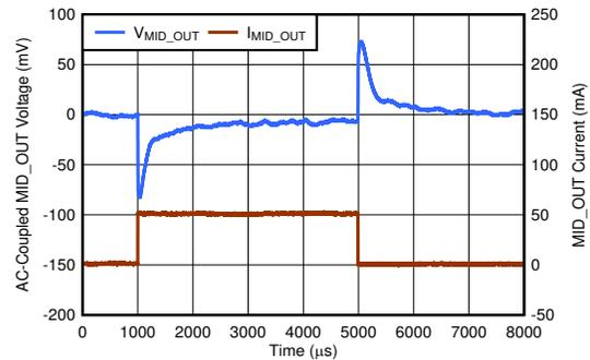
$V_{IN} = 65\text{ V}$ ,  $V_{MID\_OUT} = 12\text{ V}$ ,  $I_{MID\_OUT} = 0\text{ mA}$  to  $50\text{ mA}$  to  $0\text{ mA}$ ,
