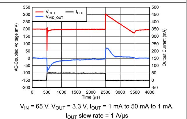
Figure 6-24. Load Transient
