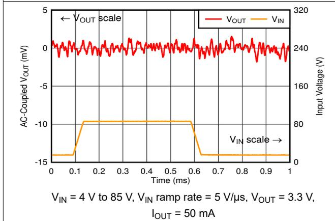
Figure 6-21. Line Transient ( $V_{MID\_OUT}$  in Dropout)
