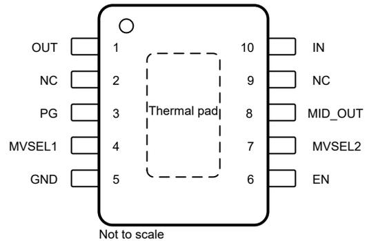
**Figure 5-2. DGQ Package (Fixed), 10-Pin HVSSOP (Top View)**
