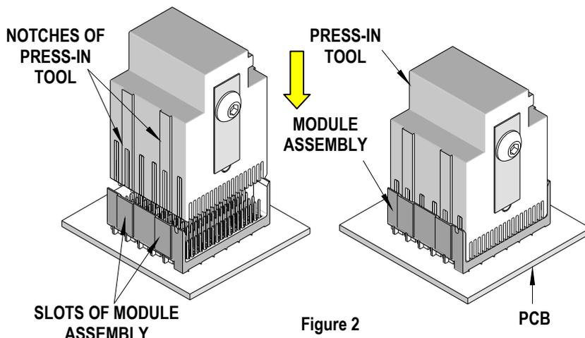
There should be no broken stand-offs along the perimeter of the part (an indication of over-pressing).
